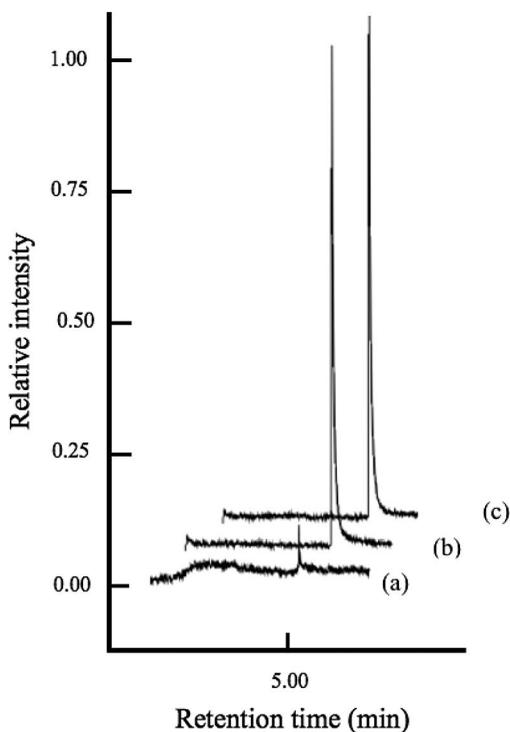
**Figure 5.** Comparison of triphenylarsine chromatograms obtained by injecting 1  $\mu\text{L}$  of 40 ppm triphenylarsine (w/v in acetone) using the direct sampling probe: (a) empty; (b) spiked on 75 mg sand; and (c) spiked on 10 mg soil.
