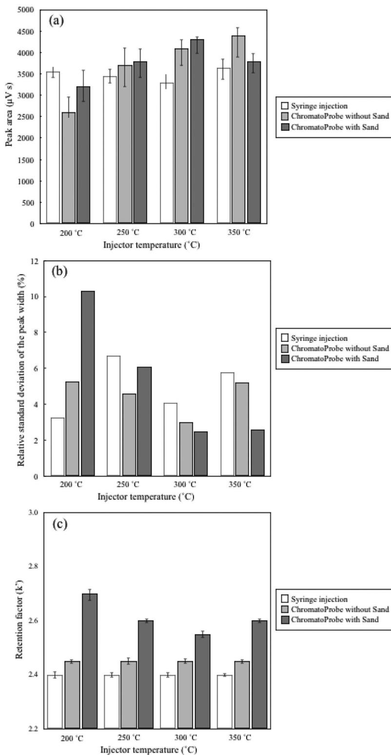
**Figure 3.** Effect of injector temperature on the triphenylarsine response for the three injection methods (syringe injection, empty sampling probe, and sampling probe with  $\sim 75$  mg of sand) using  $1.0 \mu\text{L}$  of a  $20 \text{ mg/L}$  triphenylarsine standard. Error bars are based on Student's  $t$ -value (two-tailed) at the 95% confidence interval ( $n = 3$ ).
