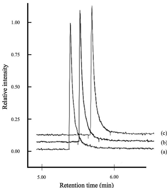
**Figure 2.** Chromatograms obtained using gas chromatography-pulsed flame photometric detection by injecting 1.0  $\mu\text{L}$  of a 20 mg/L triphenylarsine standard by use of (a) syringe, (b) empty direct sampling probe vial, and (c) direct sampling probe vial containing sand. Method conditions are described in the text.
