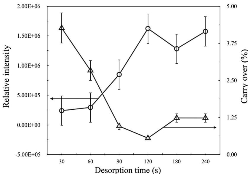
**Figure 4.** Effect of desorption time on the peak area of triphenylarsine and carryover (expressed as the percentage of peak area) using gas chromatography–mass spectrometric detection. 1.0  $\mu\text{L}$  of 40 ppm triphenylarsine was spiked on dry sand ( $\sim 100$  mg) inside of a quartz microvial. Error bars are based on Student's  $t$ -value (two-tailed) at the 95% confidence interval ( $n = 3$ ).
