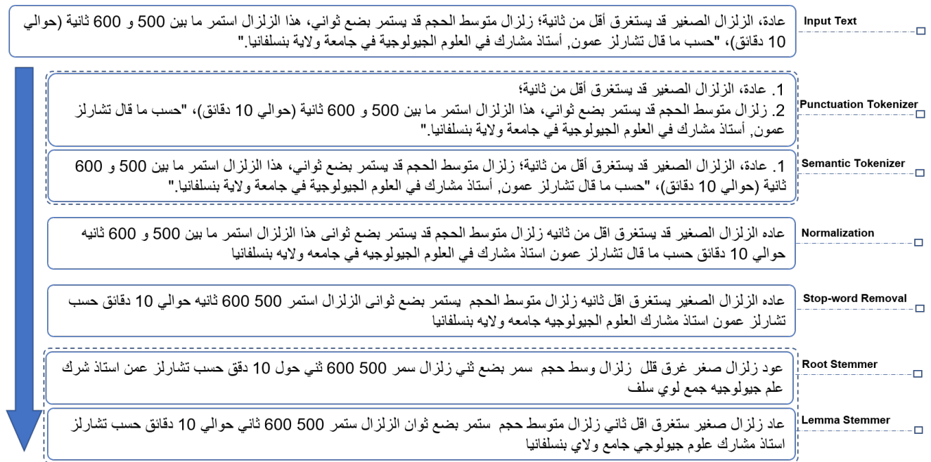
FIGURE 4. Output of text preprocessing method
