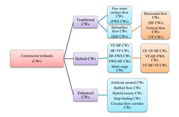
Figure 3: Classification of CWs used in wastewater treatments
