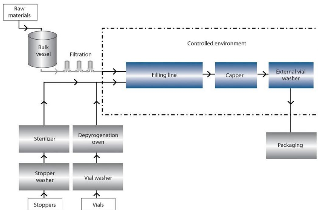
**Figure 1-3 Liquid aseptic processing**
