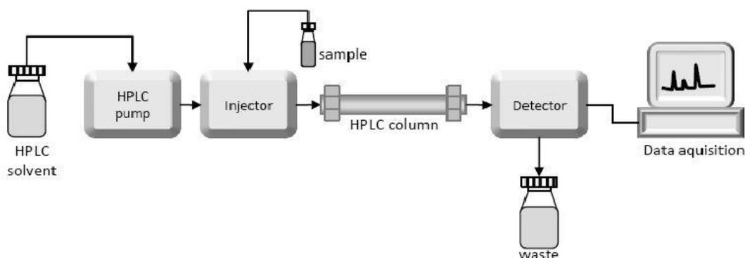
**Figure 1-6 Typical HPLC system diagram**
