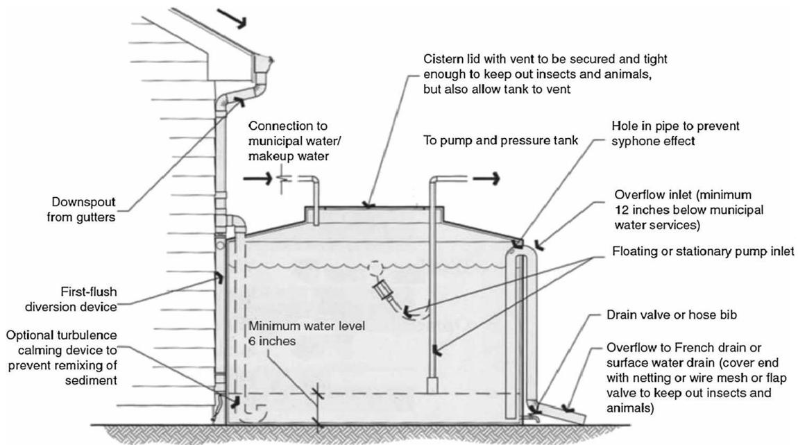
**Figure 3.2 The plumbing diagram for a rainwater harvesting system (Traboulsi and Traboulsi, 2015)**
