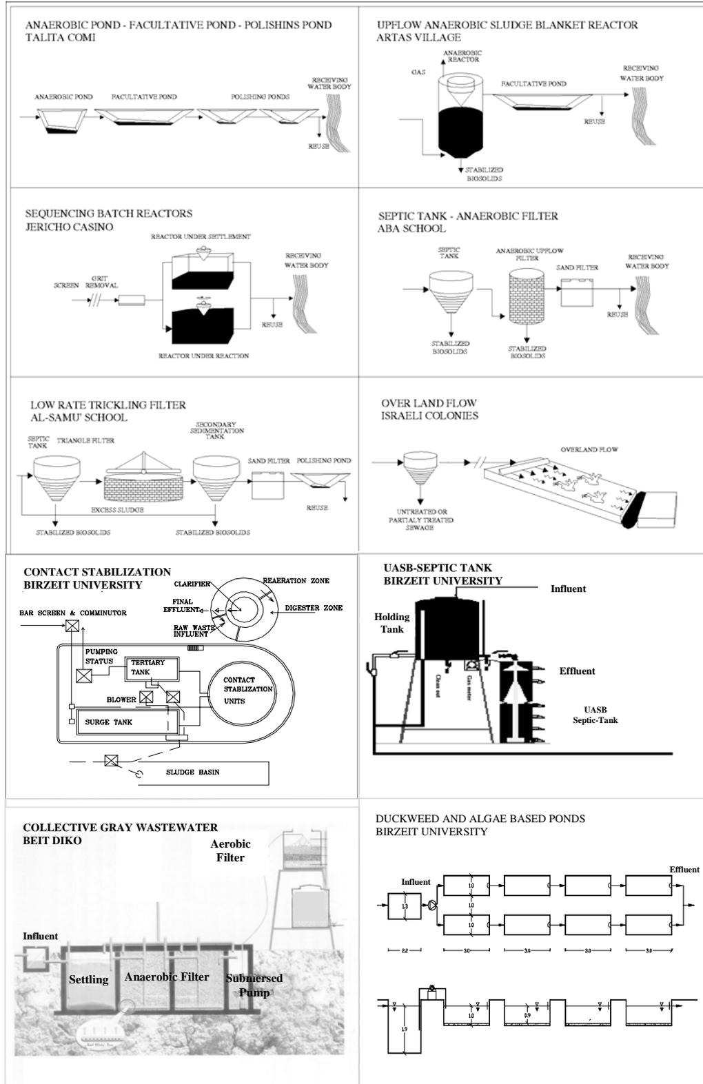
Figure 5.3: Flow sheet diagrams of onsite sewage treatment systems in rural Palestine
