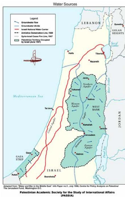
Figure 4.1: The West Bank groundwater basins and flow directions
