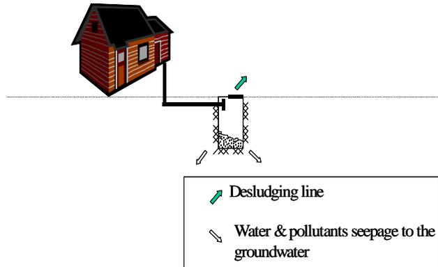
Figure 5.1: Percolation of sewage from cesspit to groundwater
