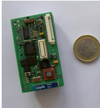
Figure 6.1: The BTnode wireless sensor node [2]
