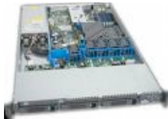
Figure 24: INTEL SR1500 Server
