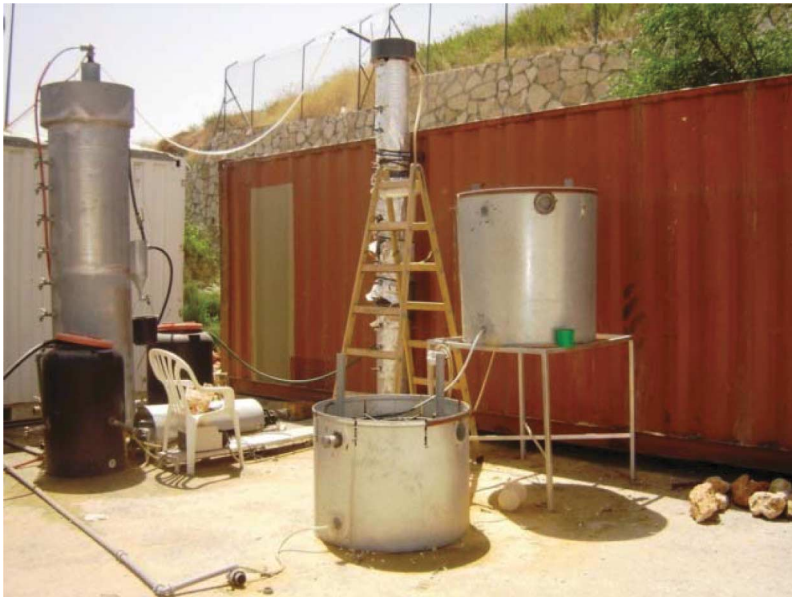
Figure 3. Post-treatment of anaerobically treated effluent using biofilters.
