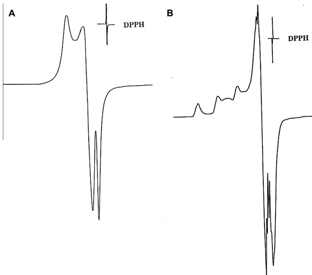
Fig. 1. X-band ESR spectrum of  $[\text{Cu}(2\text{-MeIm})_3(\text{sal})](2)$  as: (A) powder at room temperature and (B) frozen solution at  $-196^\circ\text{C}$ .
