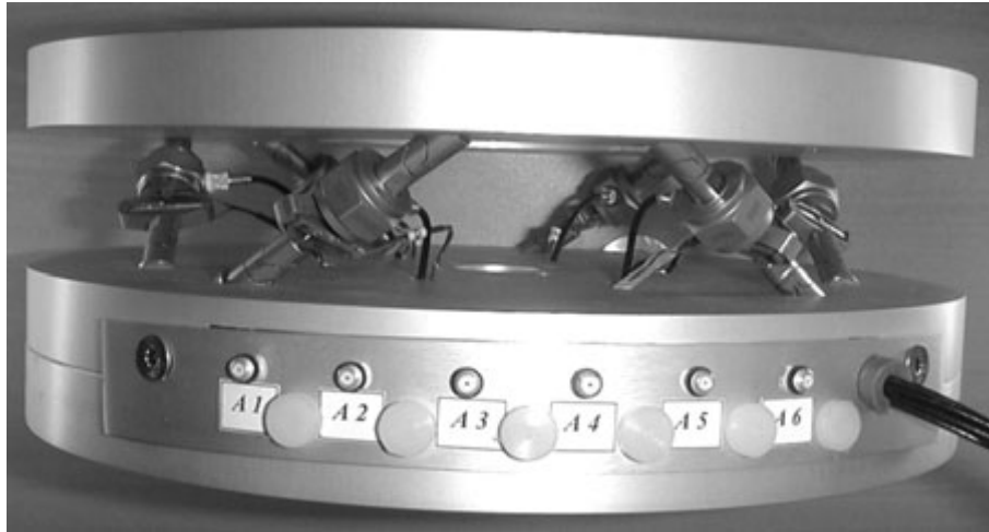
Figure 1.12: The ULB generic active damping interface
