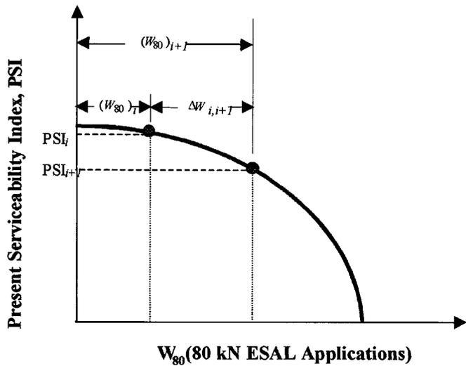
Fig. 2. Basic pavement performance curve
