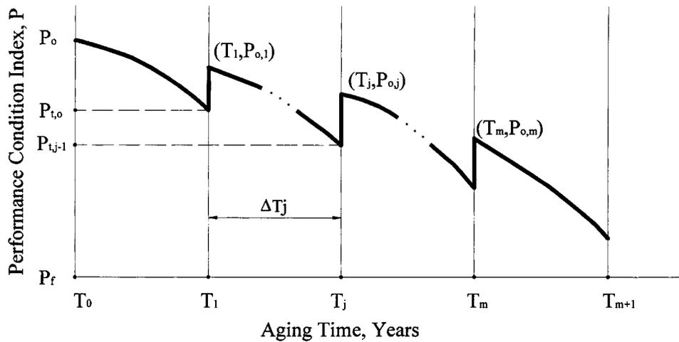
Fig. 1. Typical pavement life-cycle performance curve
