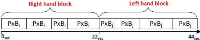
Figure 7. Motion task divided into eight sub-blocks. Where,  $\mathbf{P}$  has the value 3, 5, or 7.  $\mathbf{B}_i$  is the button number ranged from 0 to 3.  $\mathbf{B}_j$  is the button number ranged from 4 to 7.
