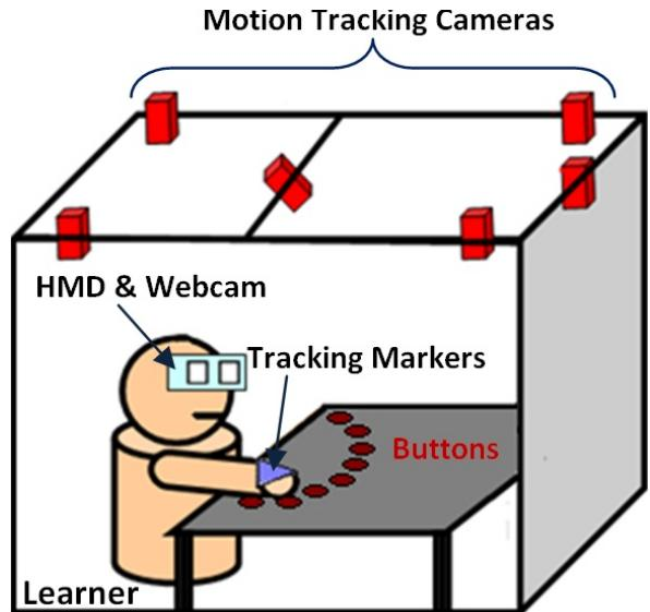
Figure 1. The physical workspace of the physical task learning support system.
