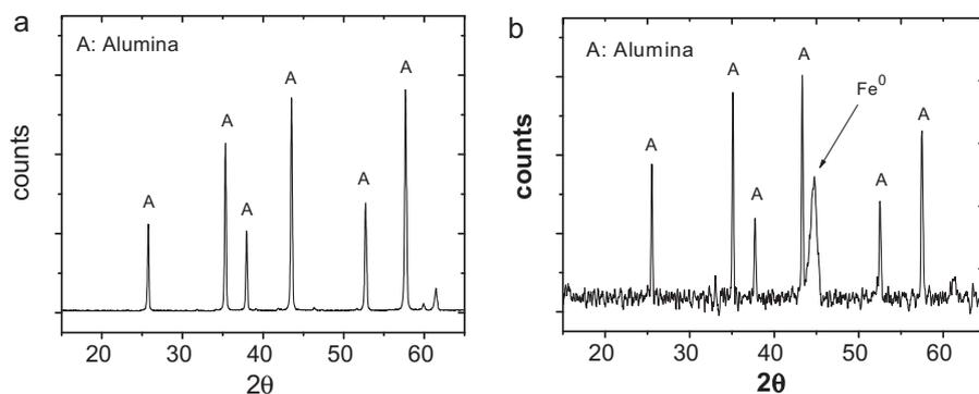
Fig. 1. XRD patterns of: (a) alumina, (b) Al-nZVI.
