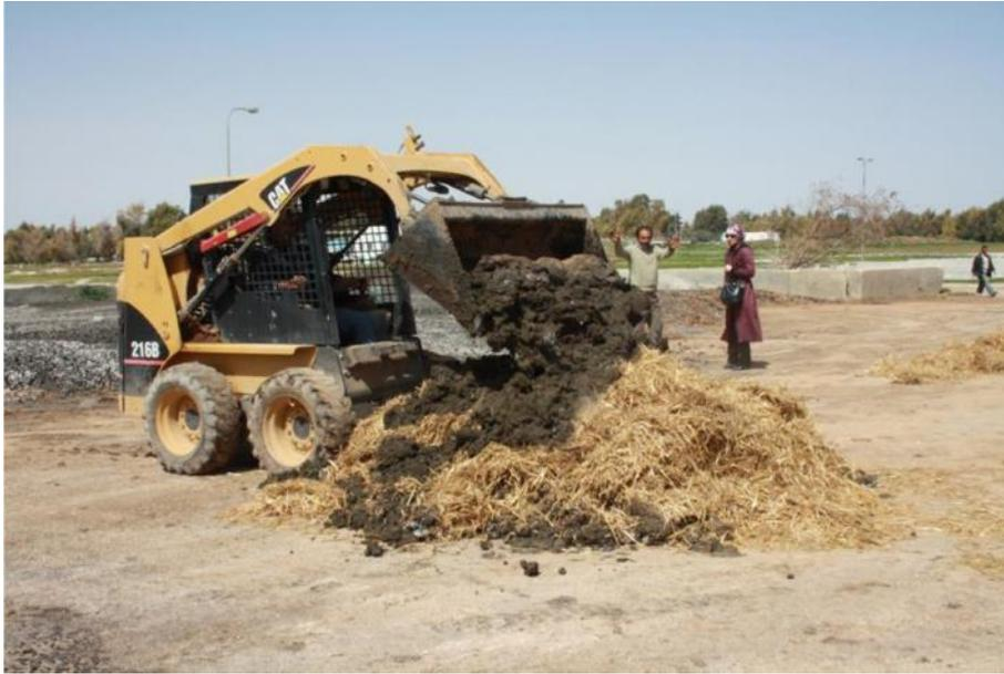
Figure 5: Piling up dewatered sludge with straw 50:50
