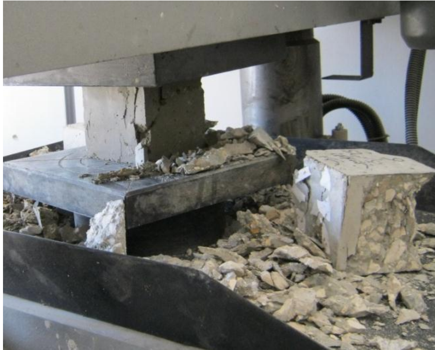
Figure 29 | Concrete block fracture and failure under pressure
