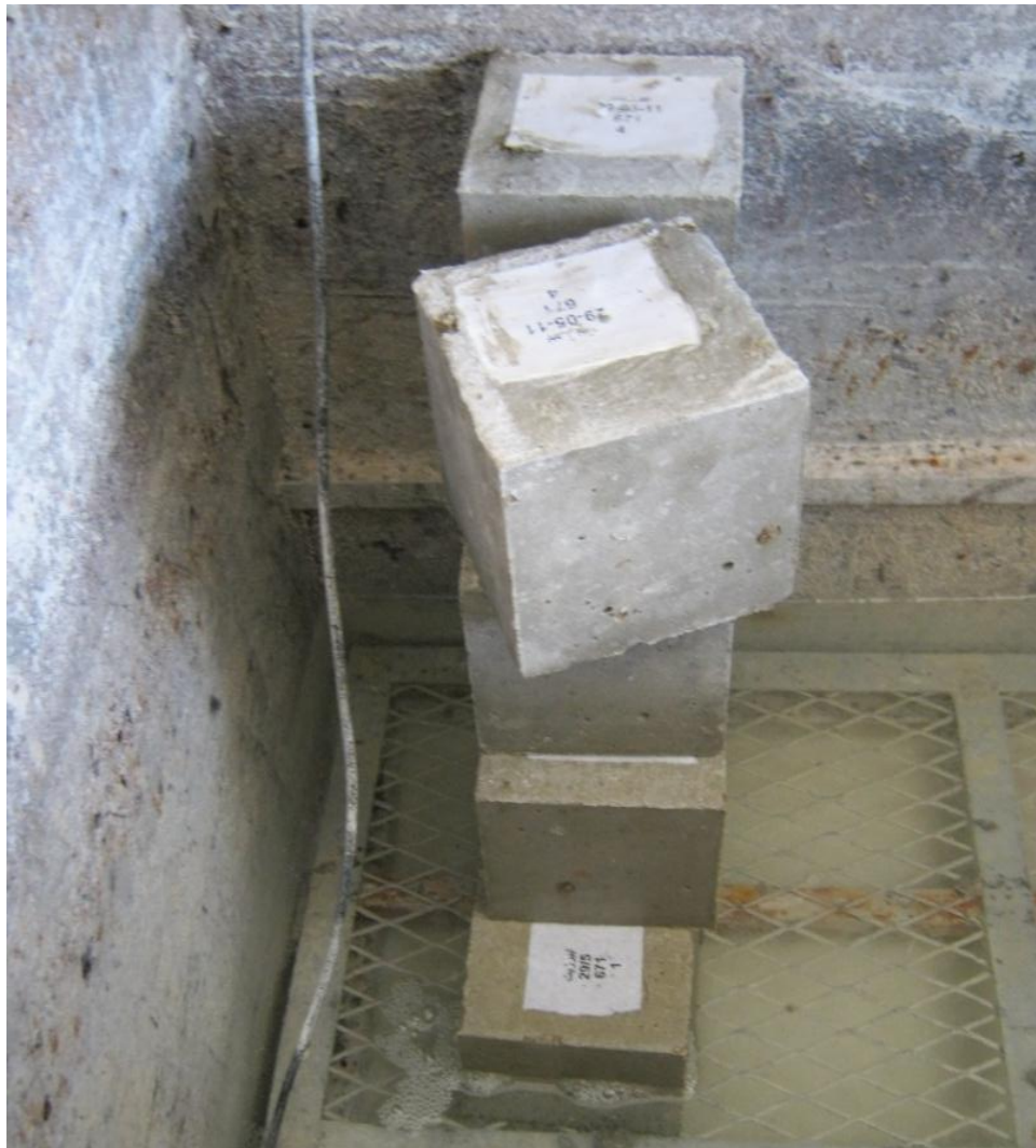
Figure 25 | Biosolids-amended specimens (10 x 10 x 10 cm blocks) are being taken placed in a water curing bath
