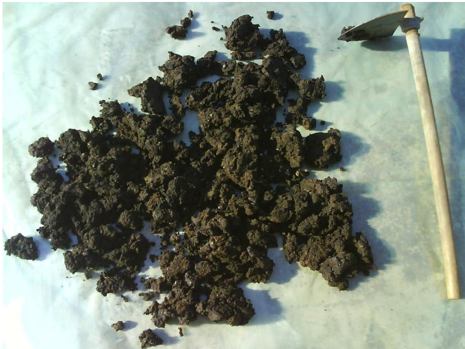
Figure 12 | Dewatered sewage sludge sample on solar-drying bed
