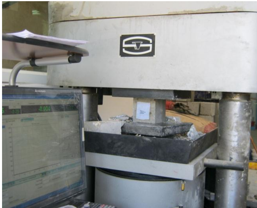
Figure 28 | Computerized testing of compressive strength of biosolids-amended specimens
