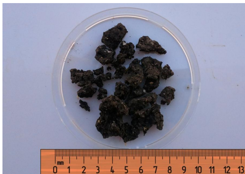
Figure 14 | Solar-dried wastewater sewage sludge
