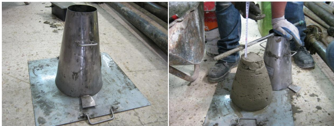
Figure 23 | Consistence tolerance testing for biosolids-amended concrete mix (lab images)
