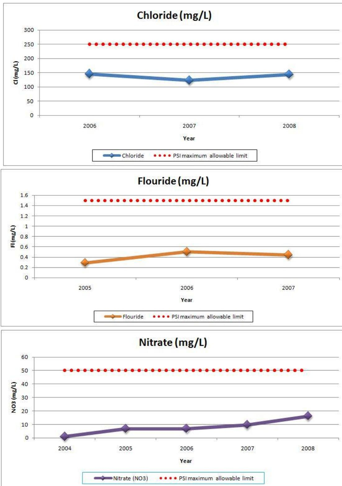
Figure 5-2 Major chemical and physical parameters measured in the network
