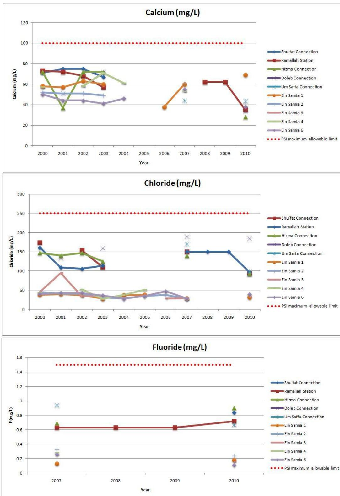
Figure 5-1 Major chemical and physical parameters measured at the sources
