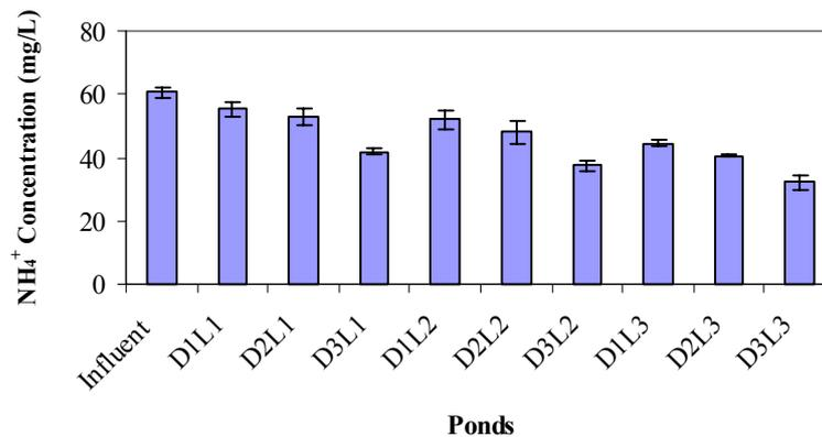
**Fig. 4.13**, Average values of  $\text{NH}_4^+$  concentration in the influent and effluent of the nine ponds of the pilot plant of DBPs (represented by the columns). The bars represent the standard error ( $\pm\sigma/n^{1/2}$ ).
