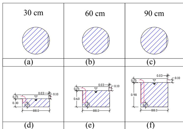
**Fig. 3.2** Top view for the ponds of depth 30, 60, and 90 cm, respectively (a,b and c) and the dimensions of the above mentioned ponds(d,e and f). All dimensions are in meter otherwise mentioned.
