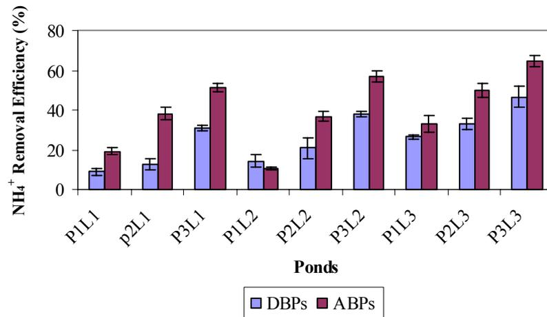
**Fig. 4.15.** Average values for the removal efficiencies (%) of  $\text{NH}_4^+$  in the nine ponds of the two experimental periods. The vertical columns represent the average values  $\text{NH}_4^+$  removal. The bars represent the standard error ( $\pm\sigma/n^{1/2}$ ).
