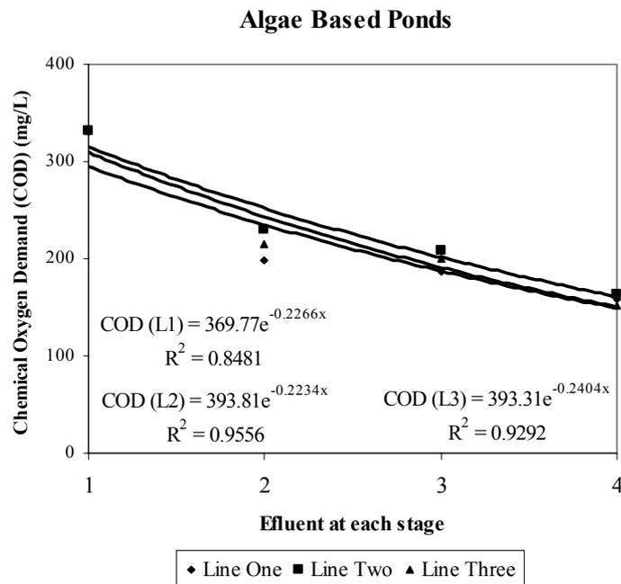
**Fig. A.2** Removal curve of COD for the three lines (90, 60, and 30 cm depth ponds) in DBPs (a), and ABPs (b). The figure shows also the best-fit exponential curve and equation for each line with the correlation coefficient between actual points and the curve. Points 1, 2, 3 and 4 (x-axis) represent influent, first, second and third ponds, respectively.
