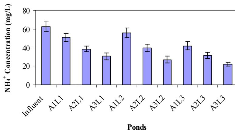
**Fig. 4.14.** The average values of  $\text{NH}_4^+$  concentration in the influent and effluent of the nine ABPs (mg/L). The bars represent the standard error ( $\pm\sigma/n^{1/2}$ ) at a level of significance  $p \leq 0.05$ .
