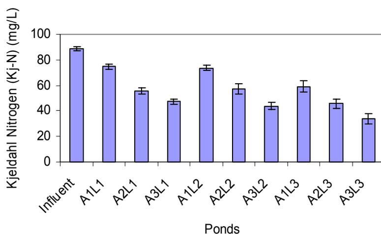
**Fig. 4.17.** Average values of TKN concentration in the influent and effluent of the nine ABPs. The error bars represent the standard error ( $\pm\sigma/n^{1/2}$ ) at a level of significance  $\rho \leq 0.05$ .
