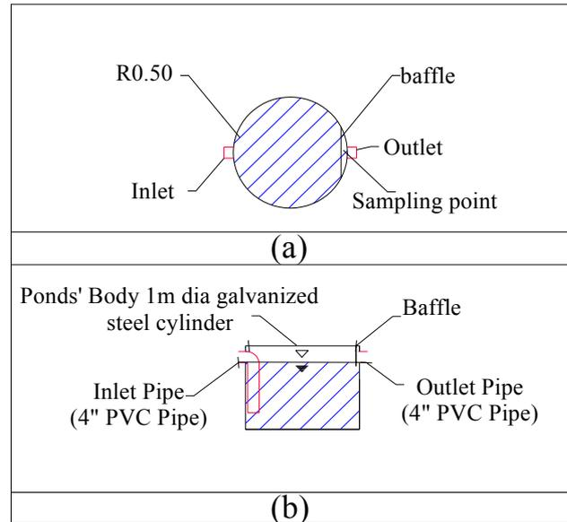
**Fig. 3.3** Schematic diagram for a typical stabilization pond; (a) shows the top view and (b) shows a longitudinal cross section for the pond.
