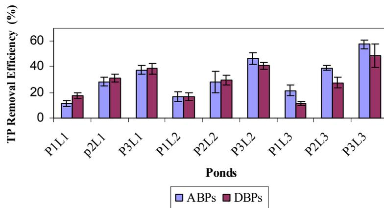
**Fig. 4.12.** Average values for the removal efficiencies (%) of TP in the nine ponds of the two periods. The vertical columns represent the average values TP removal. The bars represent the standard error ( $\pm\sigma/n^{1/2}$ ) at a level of significance  $\rho \leq 0.05$ .
