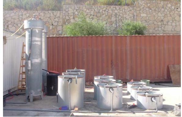
**Photo A.2.** Front view for the experimental pilot plant; the three lines of stabilization ponds and the UASB-septic tanks in AWWTP.
