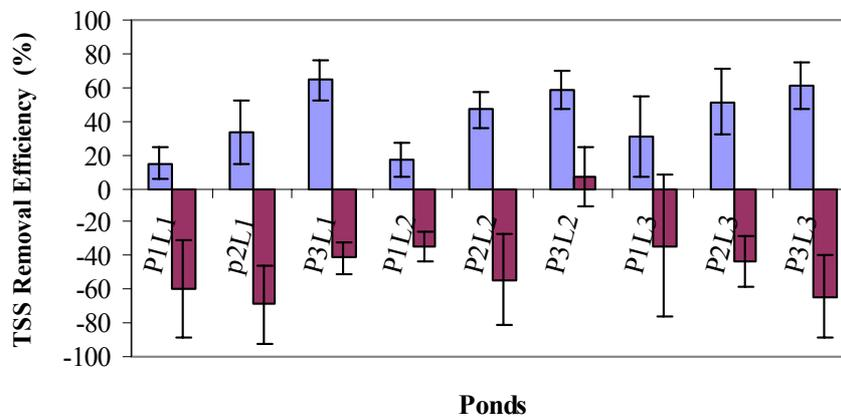
**Fig.4.5.** Average values for the removal efficiencies of TSS in the nine ponds of the two experimental periods. The vertical columns represent the average values TSS removal efficiency. The bars represent the standard error ( $\pm\sigma/n^{1/2}$ ) at a level of significance  $p \leq 0.05$ .
