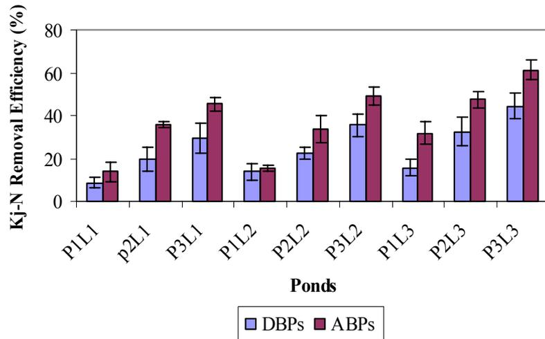
**Fig. 4.18.** Average values for the removal efficiencies (%) of TKN in the nine ponds of the two periods. The vertical bars represent the average values TKN removal. The bars represent the standard error ( $\pm\sigma/n^{1/2}$ ) at a confidence level.
