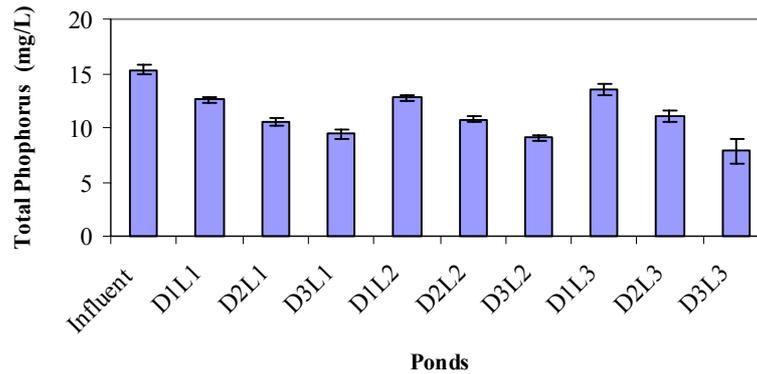
**Fig. 4.10.** The average value of TP removal efficiency in DBPs and the standard error bars ( $\pm\sigma/n^{1/2}$ ) at a confidence level of 95%.
