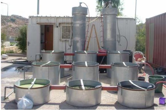
**Photo A.1.** Side view for the experimental pilot plant; the three lines of stabilization ponds and the UASB-septic tanks in AWWTP.
