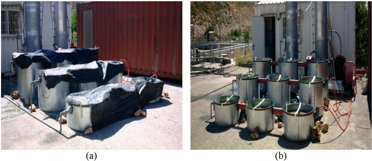
**Photo 4.1.** a- The covered ponds (five days per week). b- Cover removal (for two days per week).
