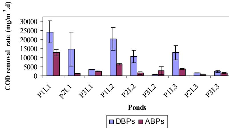
**Fig. 4.9.** Average values for COD removal rates ( $\text{mg}/\text{m}^2 \cdot \text{d}$ ) for the nine ponds in the two periods. The vertical columns represent the average values COD removal rates. The bars represent the standard error ( $\pm\sigma/n^{1/2}$ ).
