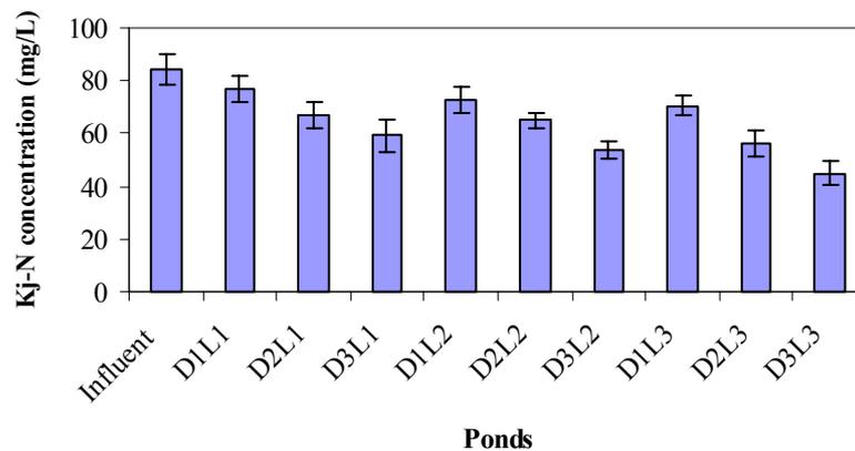
**Fig. 4.16.** Average values of TKN concentration in the influent and effluent of the nine DBPs. The bars represent the standard error ( $\pm\sigma/n^{1/2}$ ).
