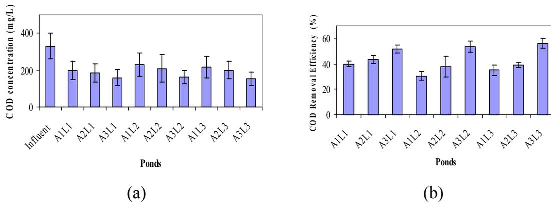
**Fig. 4.8.** Average values of COD concentration at the influent and effluent of ABPs (a) and COD removal efficiency from the nine ABPs (b). The vertical columns represent the average values for COD concentration in the influent and the nine ponds of the pilot plant, the bars represent the standard error.
