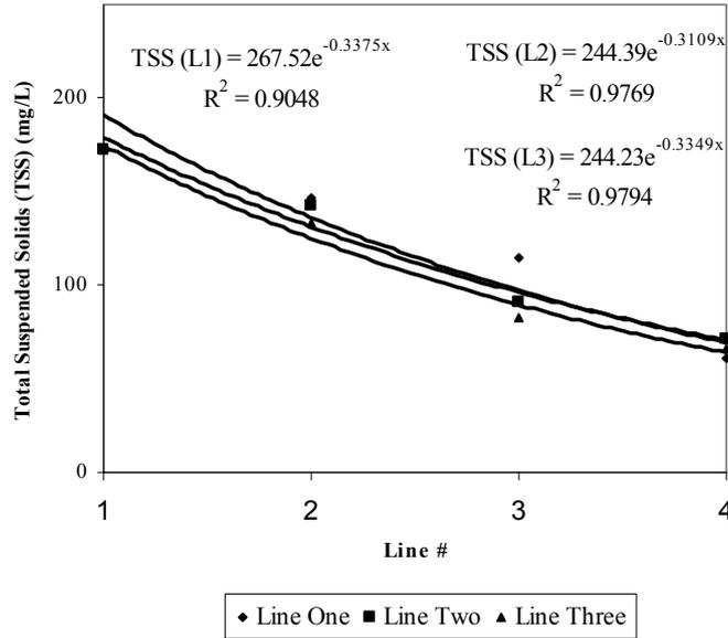
**Fig. A.6.** Removal curve of TS from the three lines (90, 60, and 30 cm depth) in ABPs. The figure shows also the best-fit exponential curve and equation for each line with the correlation coefficient between actual points and the curve. Points 1, 2, 3 and 4 (x-axis) represent influent, first, second and third ponds, respectively.
