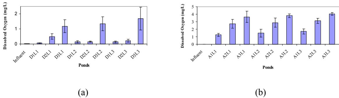
**Fig. 4.2.** DO concentration in DBPs (a) and ABPs (b). The vertical columns represent the average DO concentration in the nine ponds effluent (mg/L); the bars represent the standard error ( $\pm\sigma/n^{1/2}$ ). D stands for duckweed and A stands for algae. Note that (D or A) $iL_j$  means the  $i^{\text{th}}$  (D or A) pond in the  $j^{\text{th}}$  line (e.g.  $D_3L_1$ , means the third DBP in the first line).
