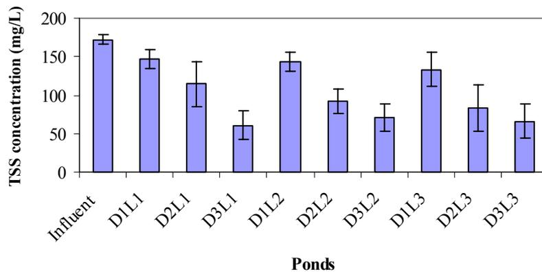
**Fig. 4.4.** The average values of TSS concentration in the influent and effluent of DBPs,  $n = 5$ . The vertical columns represent the average TSS concentration values for the influent and the nine ponds of the pilot plant, the bars represent the standard error ( $\pm\sigma/n^{1/2}$ ) at a level of significance  $p \leq 0.05$ .
