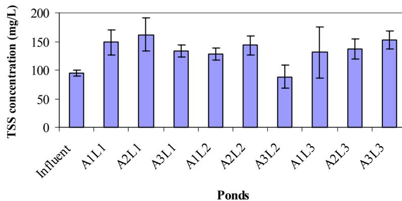
**Fig. 4.5.** The average values of TSS concentration in the influent and effluent of ABPs,  $n = 5$ . The vertical columns represent the average TSS concentration values for the influent and the nine ponds of the pilot plant. The bars represent the standard error at a level of significance  $p \leq 0.05$ .
