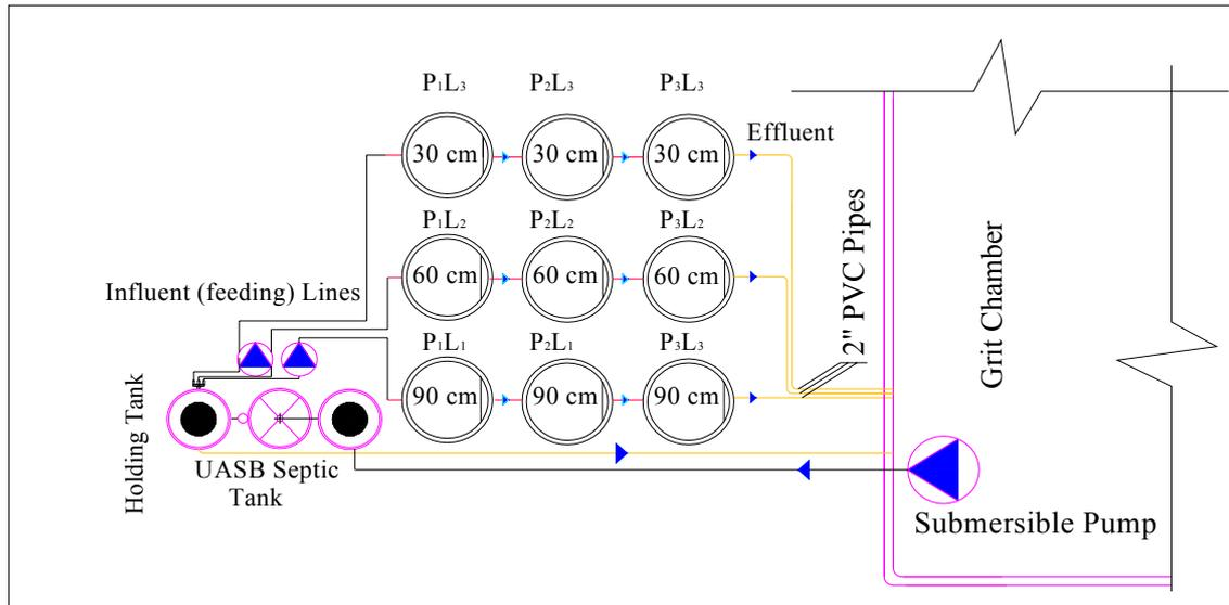
**Fig. 3.1** Schematic diagram for the stabilization ponds based pilot treatment plant; the figure shows the suction location, required pumps, holding tanks, UASB-septic tank, and the three lines of stabilization ponds. The figure shows also each pond with its' corresponding code (which is used later to describe the pond) and depth.
