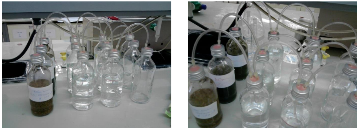
Figure 3-4: Biochemical methane potential tests; the laboratory sets
