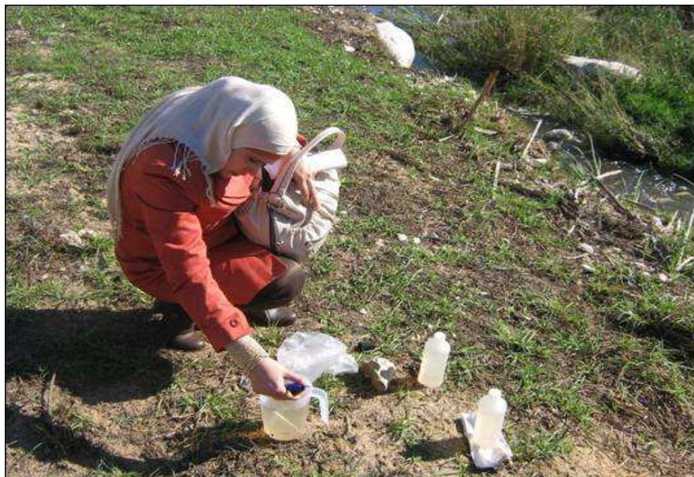
**Figure 3.3:** Measuring physical parameters in the water samples (pH, Temperature and TDS)
