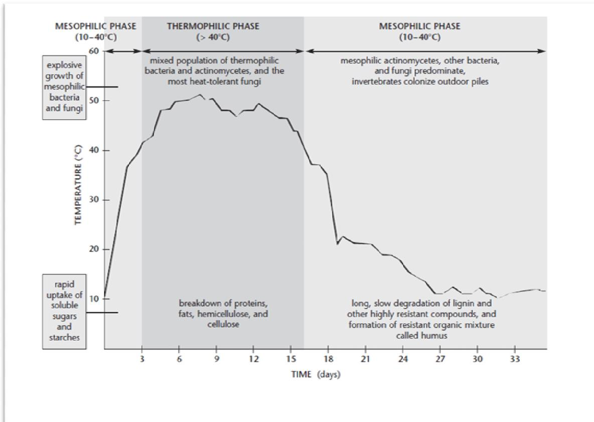
**Fig. 2.5:** Phases of thermophilic composting (Trautmann et al., 1997).
