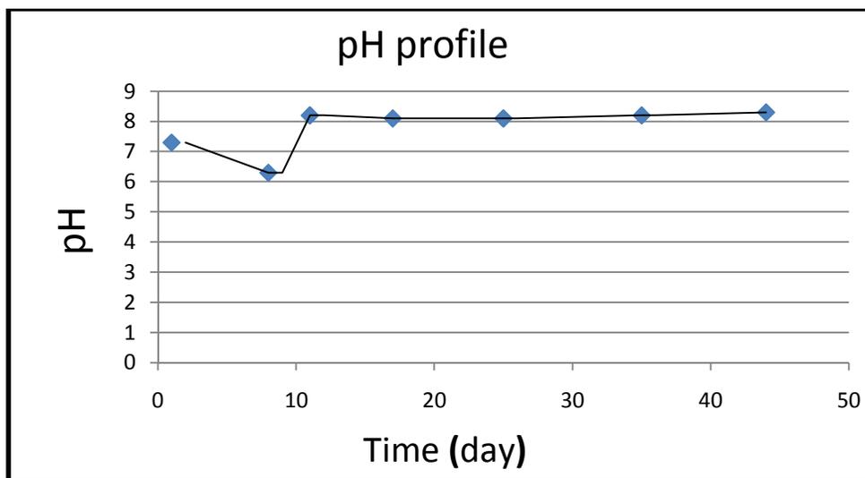
**Fig. 4.2:** pH variations during the composting process.
