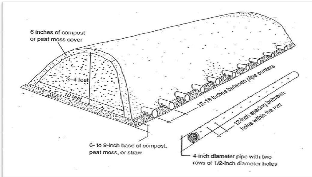
**Fig. 2.7:** Passively aerated windrow (Schneider et al., 2001).
