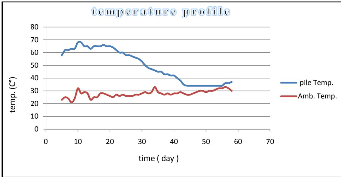
**Fig. 4.1:** Temperature variations in 40 cm depth of the pile compared to ambient temperature variations.
