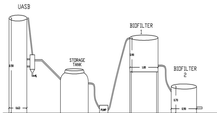
**Figure 9:** A schematic diagram of the pilot scale treatment system.
