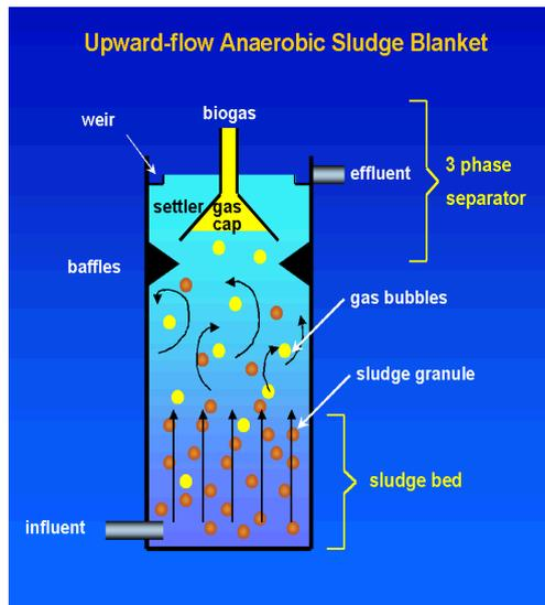
**Figure 2:** Upflow Anaerobic Sludge Blanket (UASB).
