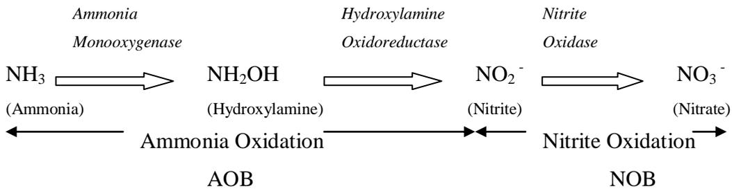
**Figure 3:** The Process of Nitrification
