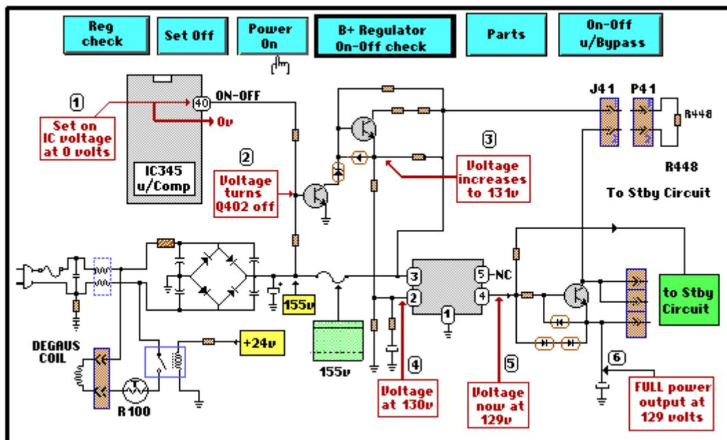
Fig 2-11 TV circuit diagram
