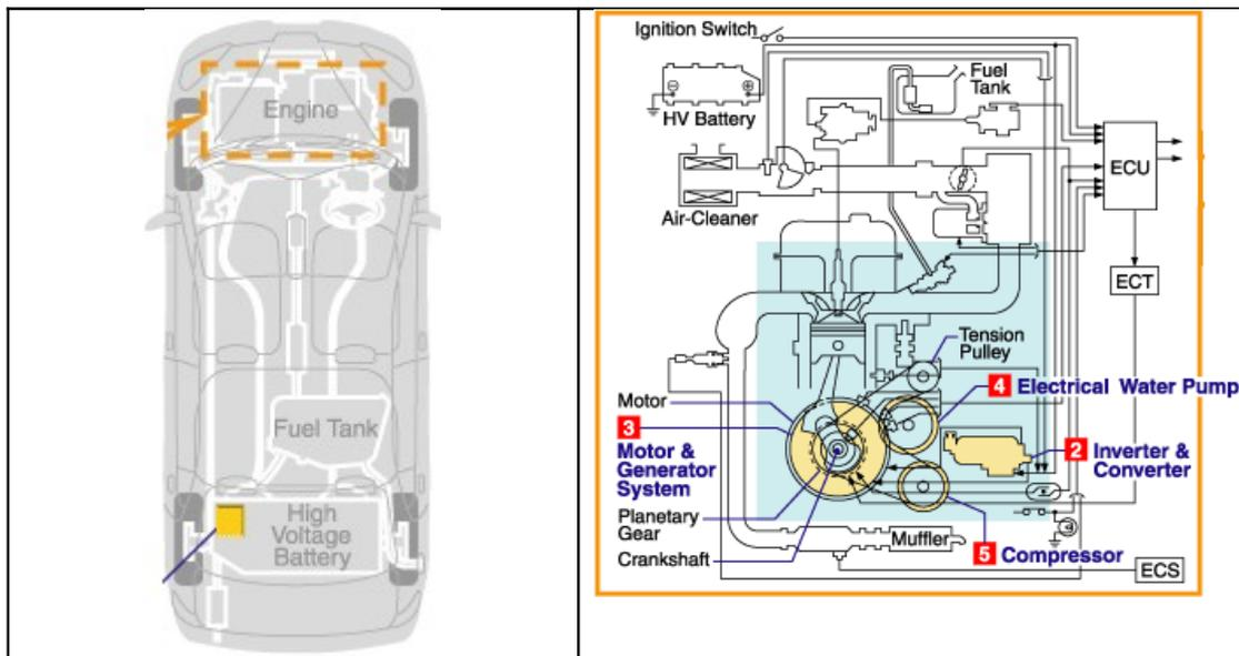
Fig 1-2 Car hybrid engine vehicle block diagram
