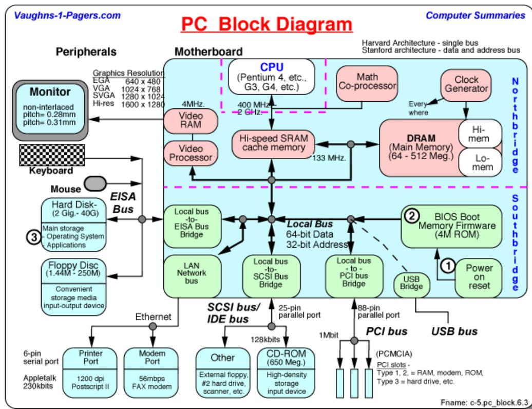
Fig 1-3 Pentium4 PC Block Diagram
