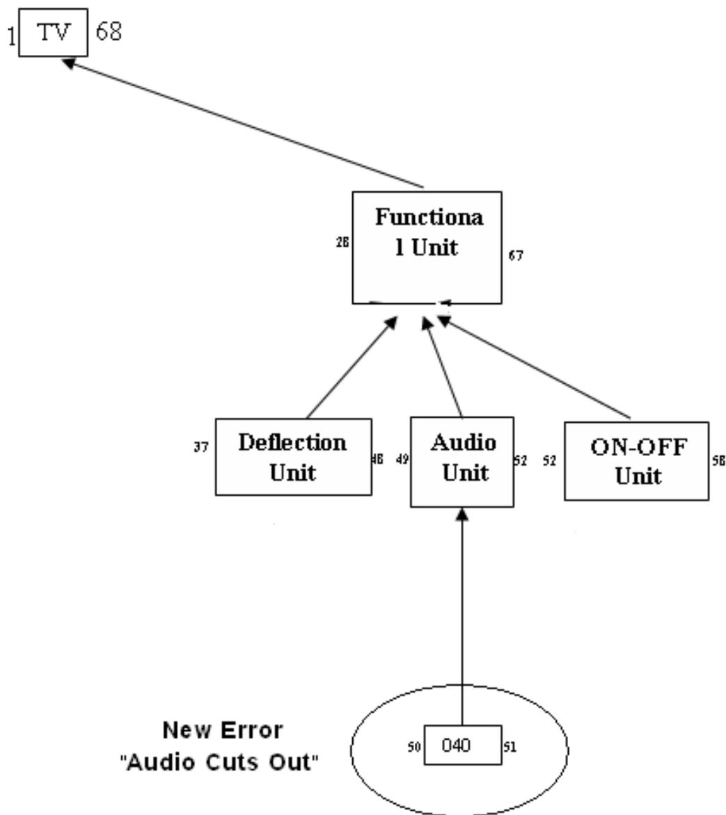
Fig 4-5 Adding new error "Audio Cuts Out" with code 040
