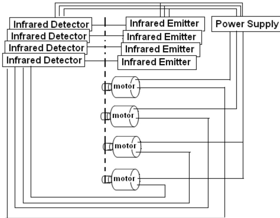
Fig 5-1: Diagram of speed control system in a robotic system
