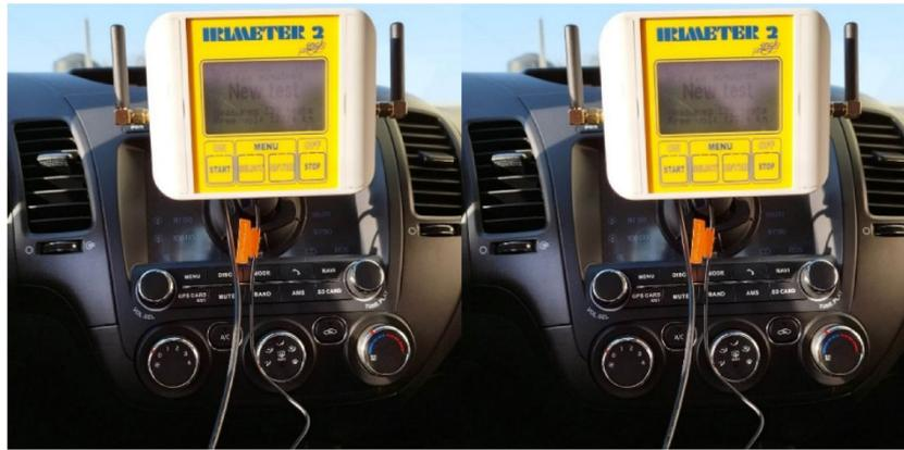
(A) Control unit with graphic LCD display mounted on vehicle dashboard.
