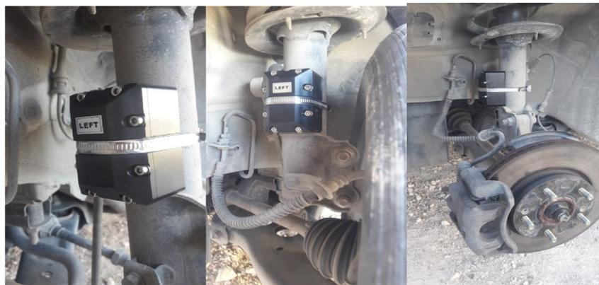
(B) Wireless inertial sensor mounted to each wheel-support assembly.
