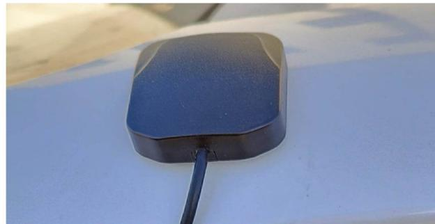
(C) Magnet GPS antenna mounted on vehicle's roof.
