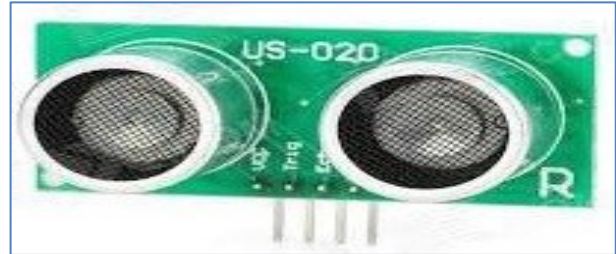
Figure 11. Physical representation of ultrasonic sensor
