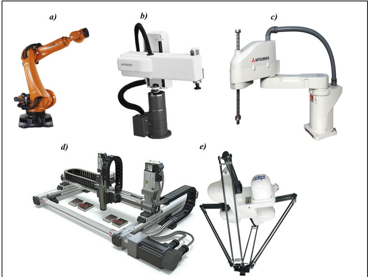
Figure 2:1: Types of the industrial robots from mechanical structure point of view: a) articulated [Kuk-16a] b) cylindrical [Den-16] c) SCARA [Mit-16] d) gantry [Pbc-16] e) parallel [ADE-16].
