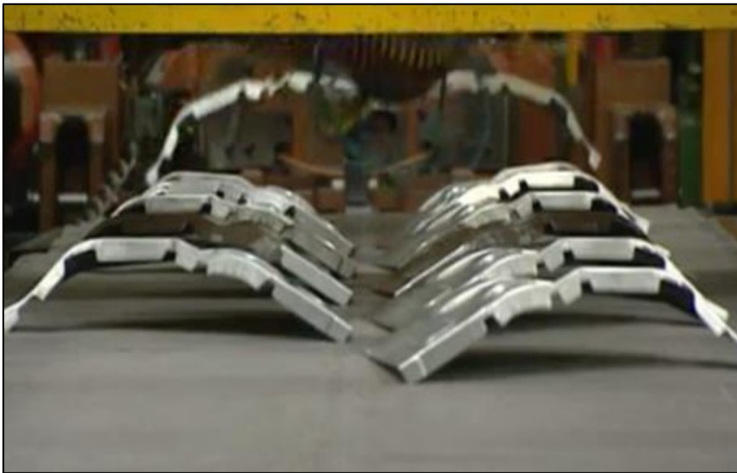
Figure 6:10: Reinforcement sheet metal used in a car.
