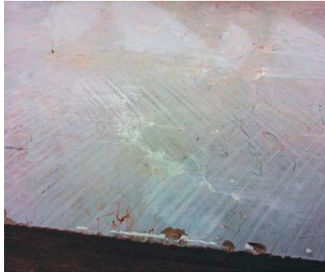
Fig. 1. Corrugation and cracks on the stone's face due to bad cutting
