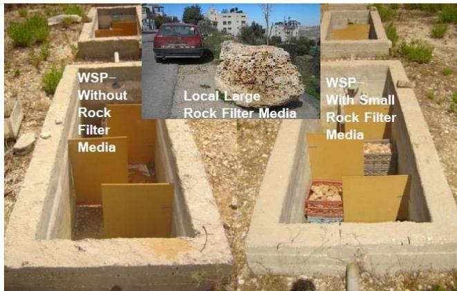
Novel design concept for facultative ponds using rock filters to reclaim the effluent. J. Environ. Eng., 2011. <http://hdl.handle.net/20.500.11889/2769>
