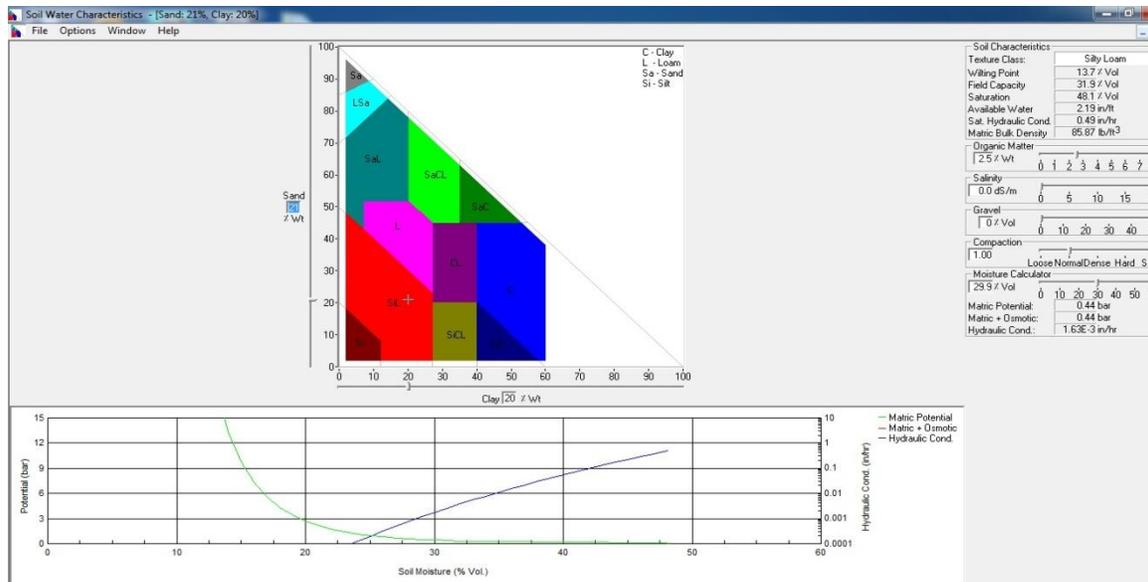
Figure 3.6: Soil water characteristics for Silt Loam soil.
