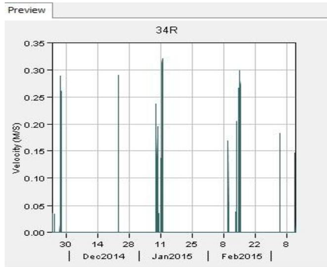
Figure 6.14: Flow velocity for reach element 34R for direct runoff from hourly model for season 2014/2015 (HEC-HMS).
