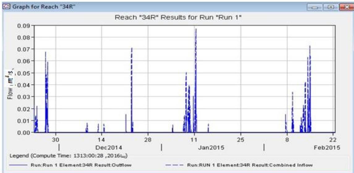
Figure 6.12: Flow for reach element 34R for direct runoff from hourly model for season 2014/2015 (HEC-HMS).
