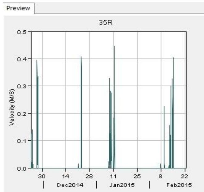
Figure 6.15: Flow velocity for reach element 35R for direct runoff from hourly model for season 2014/2015 (HEC-HMS).
