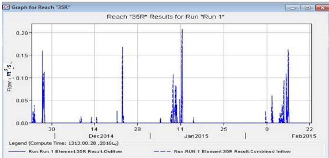
Figure 6.13: Flow for reach element 35R for direct runoff from hourly model for season 2014/2015 (HEC-HMS).
