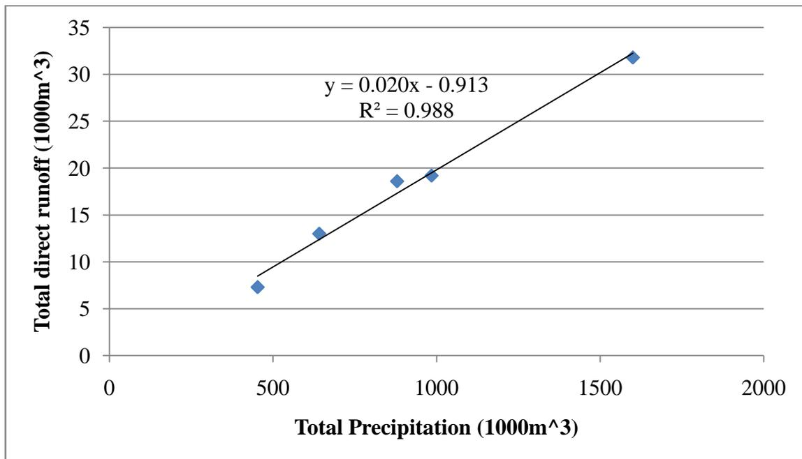
Figure 6.17: The relationship between the total amount of rainfall and the total amount of direct runoff for the five storm events.
