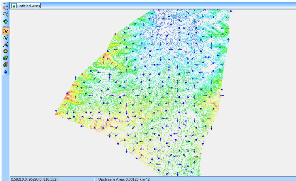
Figure 3.4: Yatta area digital elevation model, flow direction, and stream network.
