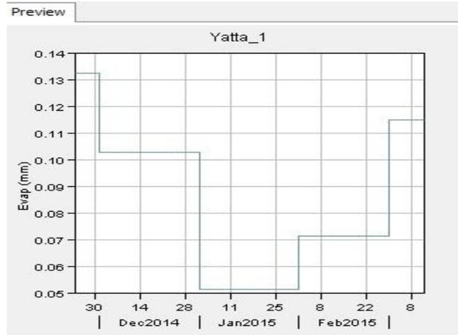
Figure 6.11: Evapo-transpiration rate for Yatta-1 subbasin for direct runoff from hourly model for season 2014/2015 (HEC-HMS).
