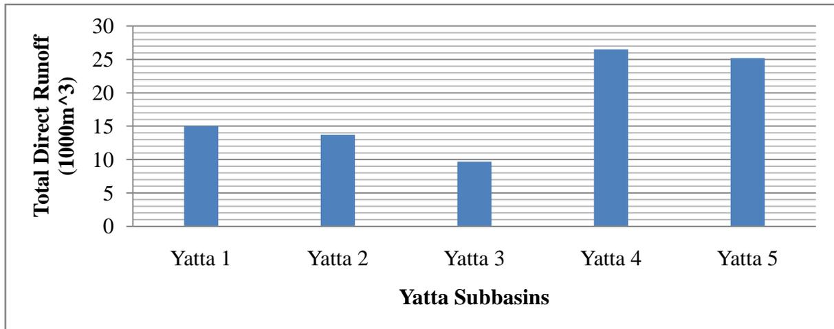
Figure 6.4: Total direct runoff for each subbasin for direct runoff from hourly model for season 2014/2015 (HEC-HMS).
