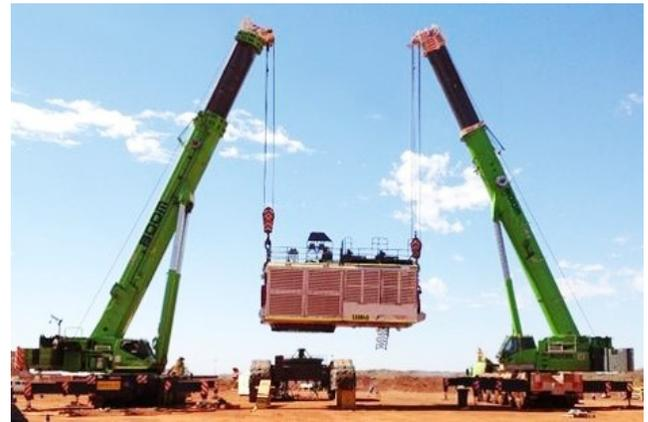
Fig. 1: Tandem-Lifting Cranes [3].
