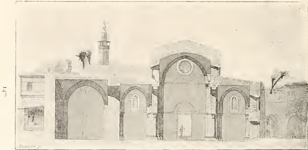
TRANSVERSE SECTION, AS YOU LOOK AT THE ENTRANCE FROM INSIDE. Scale \frac{1}{32} .
