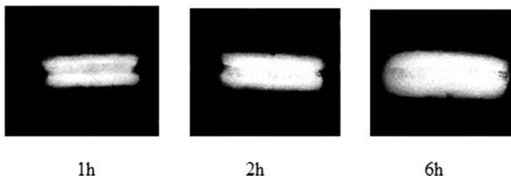
Fig. (9). Morphological changes of the three layer tablets during dissolution 1, 2 and 6 hours.
