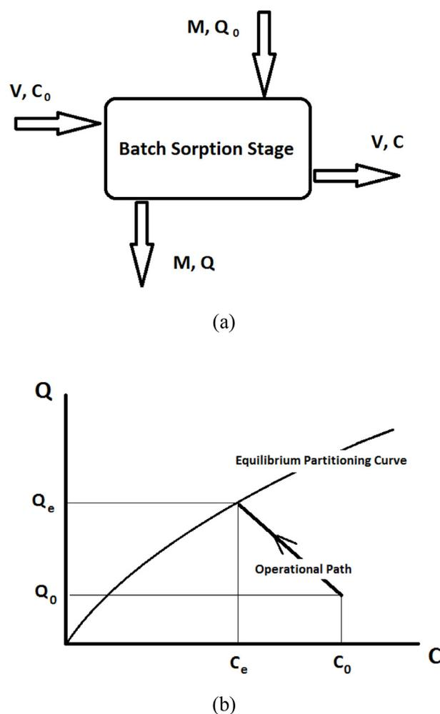
**Fig. 1.** (a) A typical schematic representation of inlet and outlet sorbate concentrations in a single stage batch sorption unit.  $C_0$  and  $Q_0$  are the initial sorbate concentrations,  $C$  and  $Q$  are the sorbate concentrations at equilibrium,  $V$  is the volume of the solution, and  $M$  is the mass of the sorbent. (b) A typical isotherm and an operational path in a single stage batch sorption operation. The slope of the operational line stands for the  $(-V/M)$  ratio.
