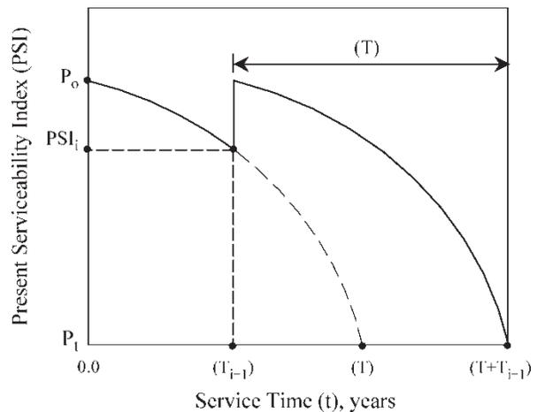
FIGURE 4 Performance curve associated with overlaid pavement.
