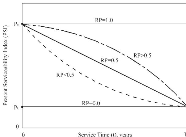
FIGURE 3 Performance curves with typical relative performance values.
