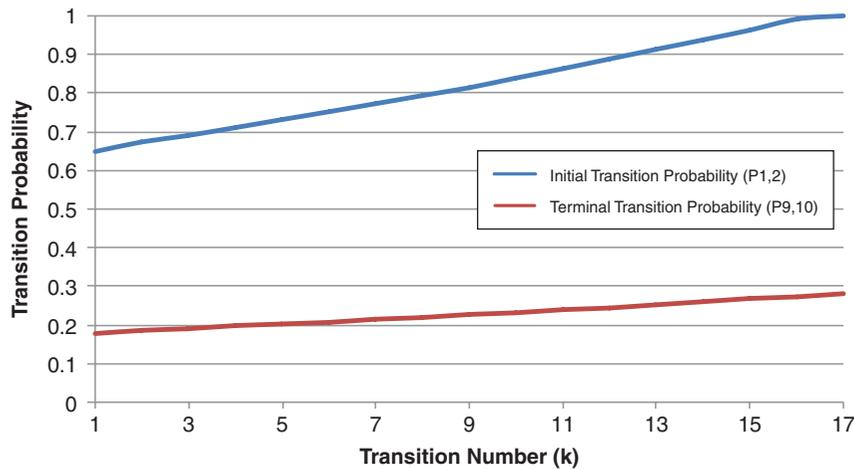
Figure 4. Sample initial and terminal transition probabilities for decreasingly lower deterioration rates ( $P_{1,2} > P_{9,10}$ ).
