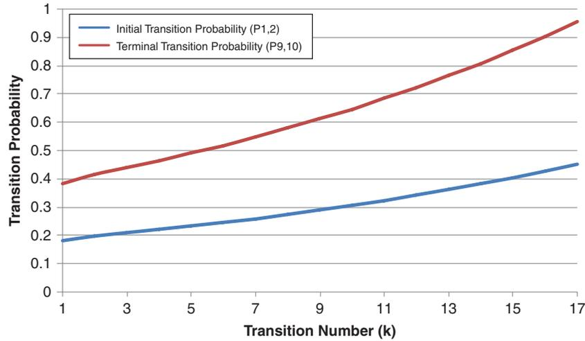
Figure 3. Sample initial and terminal transition probabilities for increasingly higher deterioration rates ( $P_{1,2} < P_{9,10}$ ).
