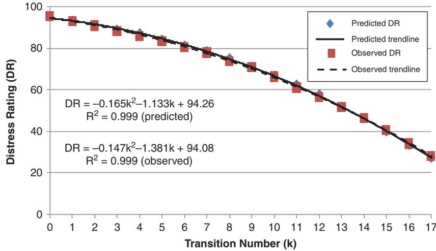
Figure 1. Sample predicted and observed pavement DRs for increasingly higher deterioration rates (i.e.  $P_{1,2} < P_{2,3} < \dots < P_{9,10}$ ).
