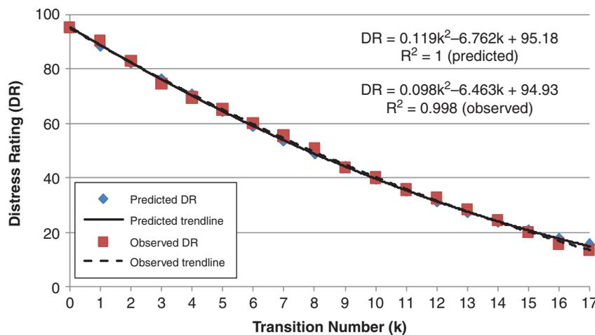
Figure 2. Sample predicted and observed pavement DRs for decreasingly lower deterioration rates (i.e.  $P_{1,2} > P_{2,3} > \dots > P_{9,10}$ ).
