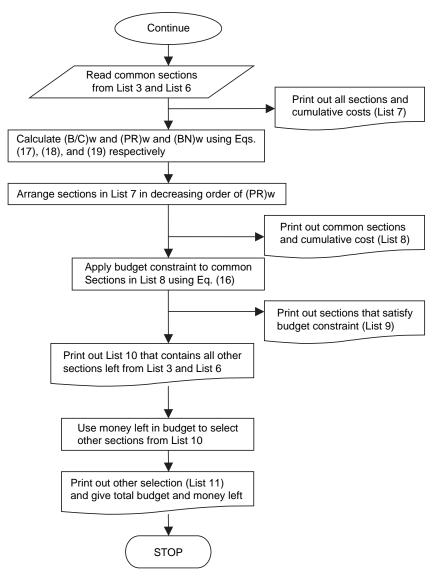
FIGURE 4 Flowchart of program logic for budget constraint.
