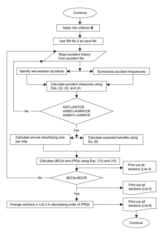
FIGURE 3 Flowchart of program logic for Risk Criterion B.
