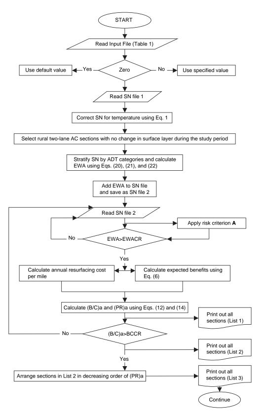
FIGURE 2 Flowchart of program logic for Risk Criterion A.
