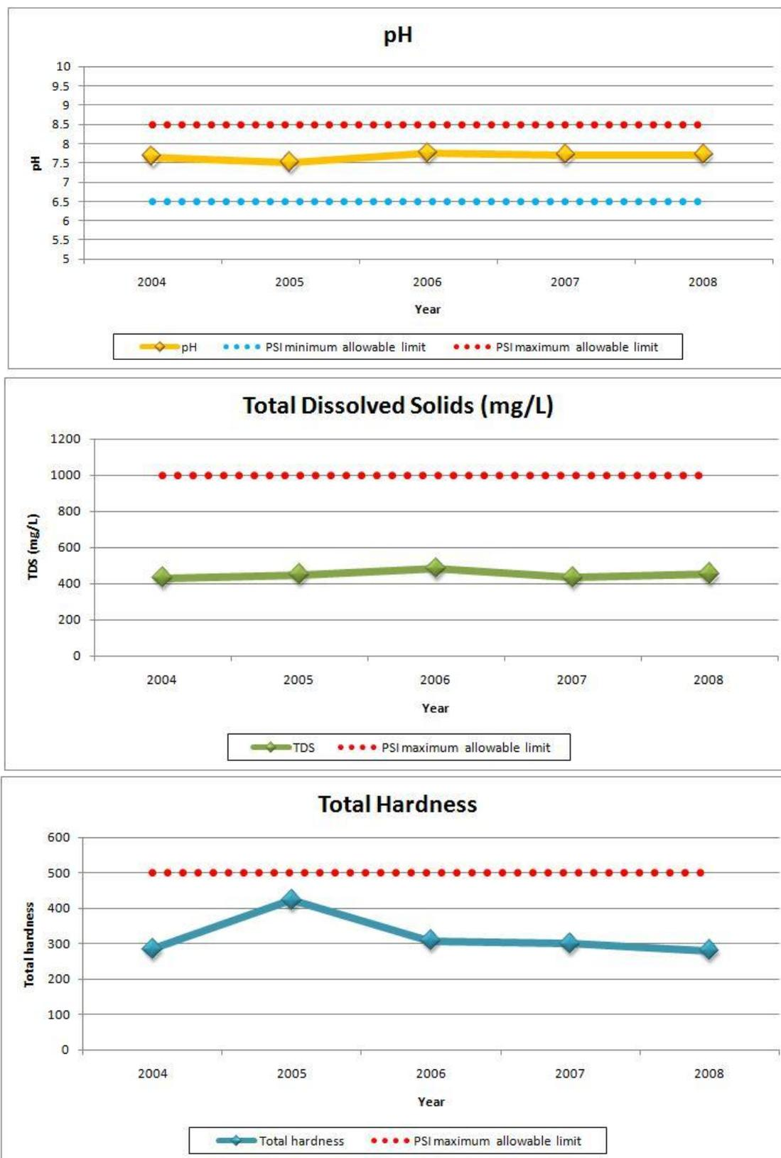
Figure 5-2 Major chemical and physical parameters measured in the network
