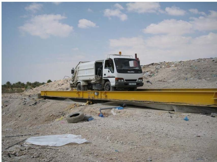
Figure 2.2: Weighing refuse compactor on the weighbridge at Jericho landfill site
