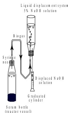
Figure 3.2. Schematic diagram of the liquid displacement setup for methane gas measurement
