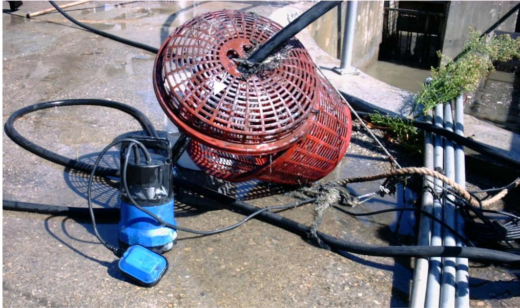
**Photo 7.** The submersible pump that was used to feed the holding tank with raw sewage from the grit removal chamber at Al-Bireh WWTP. The submersible pump was placed inside plastic basket to protect it from clogging with course materials.
