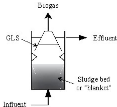
Figure 2.2. Schematic diagram of UASB reactor
