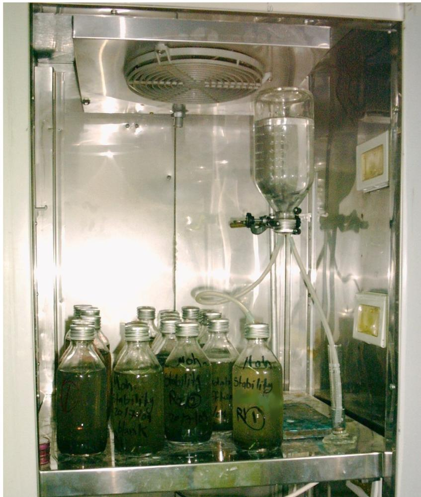
**Photo 12.** The liquid displacement set-up that used for methane gas measurements from the stability bottles inside the incubator.
