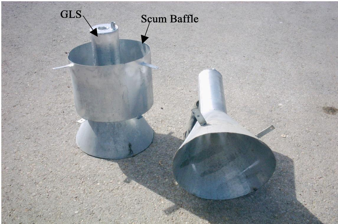
**Photo 3.** Configurations of the gas-liquid-solids phase separators (GLS) and scum baffles used inside the UASB-septic tank reactors
