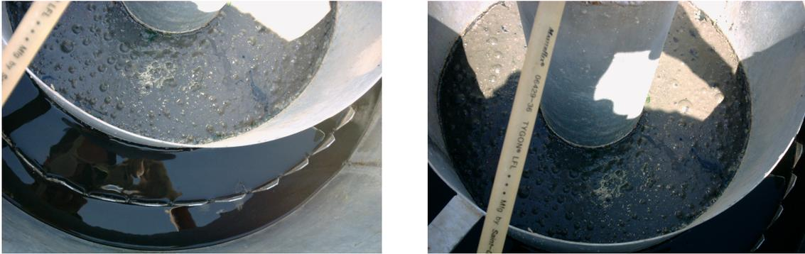
**Photo 11.** The scum layer phenomena inside the scum baffle in R1 (left) and R2 (right) at day 85 of reactors operation
