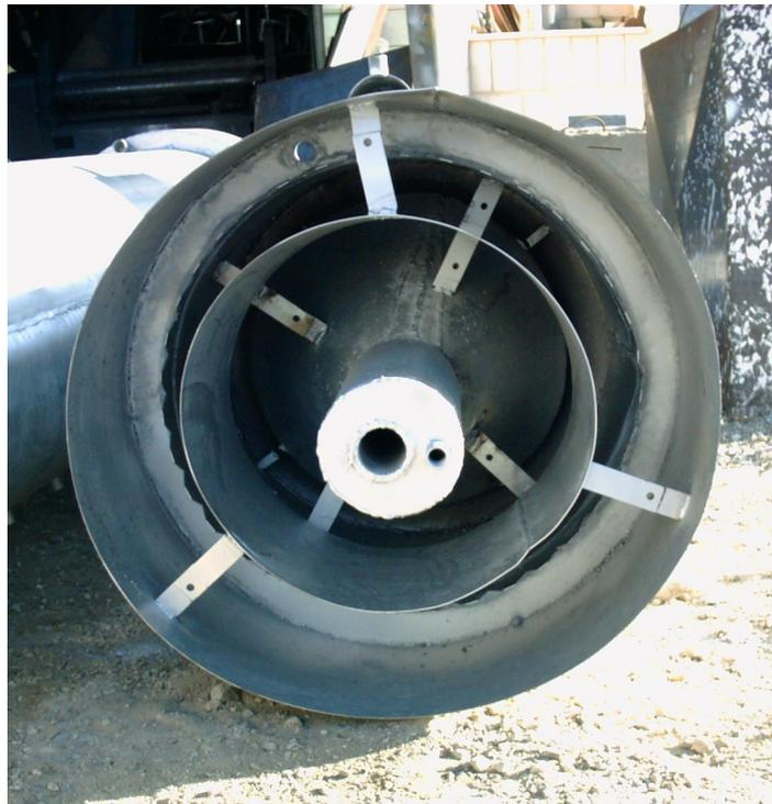
**Photo 4.** Top view of the pilot scale UASB-septic tank reactor before installation, showing the arrangement of the GLS and the scum baffle inside the reactors
