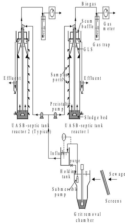
Figure 3.1. Schematic diagram of the experimental set-up (not to scale). Description of the equipments is provided in the text. GLS = Gas-liquid-solids separator; LC = Level controller
