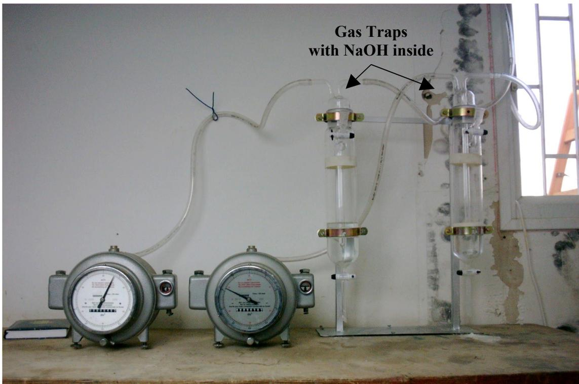
**Photo 10.** The gas meters (left) and the gas traps with 16% NaOH inside (right) that used to measure the methane gas production from the pilot scale UASB-septic tank reactors
