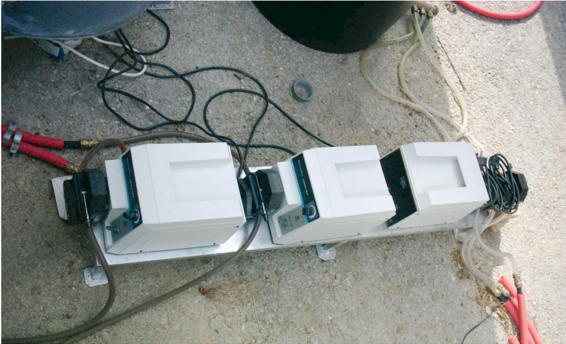
**Photo 9.** The Masterflex peristaltic pumps that were used to feed the pilot plants with raw sewage from the holding tank.
