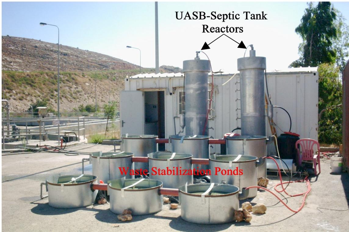
**Photo 1.** The UASB-septic tank pilot plants with waste stabilization ponds at Al-Bireh WWTP-Palestine, as an integrated treatment of raw sewage
