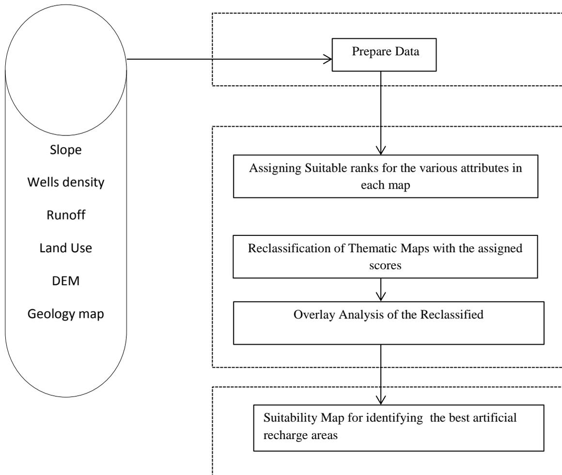
Figure 4.1: Methodology flowchart for the artificial recharge of groundwater.
