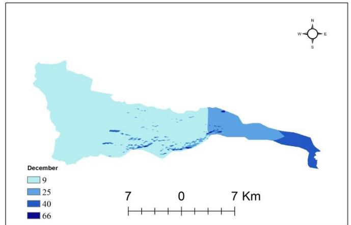
Figure 3.12: The monthly runoff (mm) in the Al-Qilt catchment.
