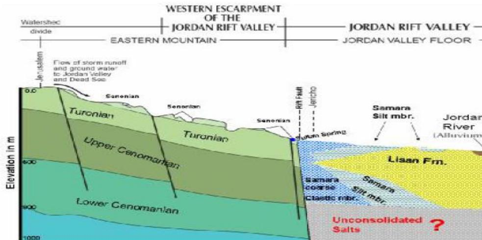
Figure 2.8: Schematic hydrogeological system in the AL-Qilt catchment. (Abu Helo, 2008).
