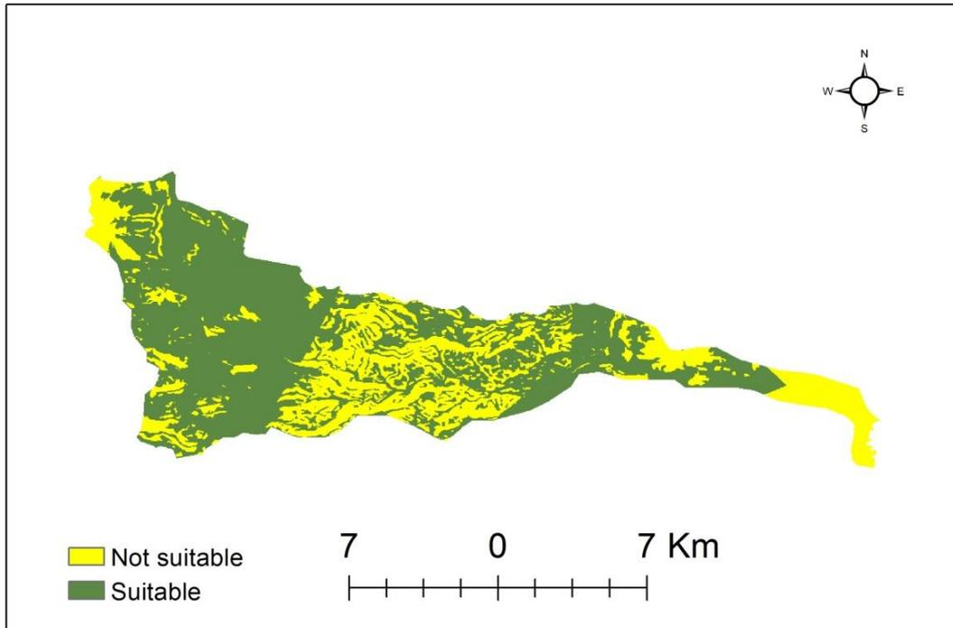
Figure 4.7: The suitability map of artificial recharge by using treated wastewater.
