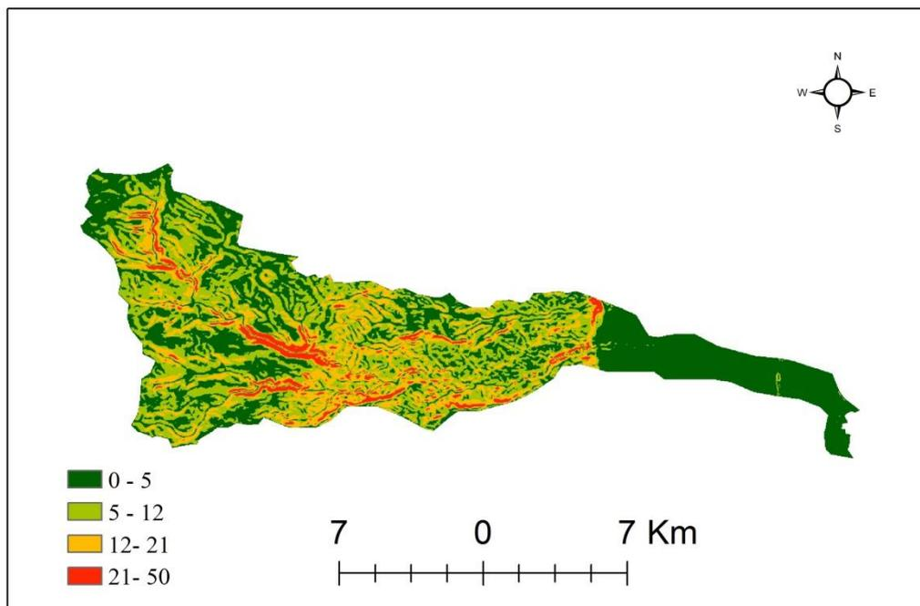
Figure 4.2: The slope in degree for Al- Qilt catchment.
