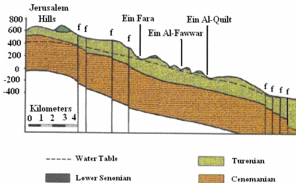
Figure 2.3: Geological sketch section along the line of springs in Al-Qilt catchment.
