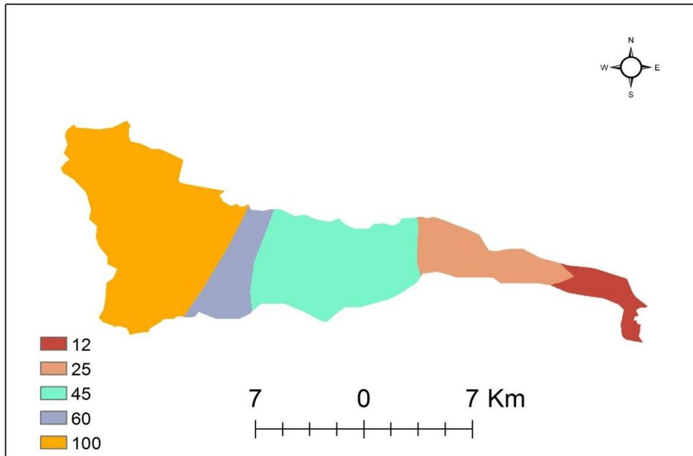
Figure 3.3: The Soil Available Water Capacity for Al-Qilt catchment .
