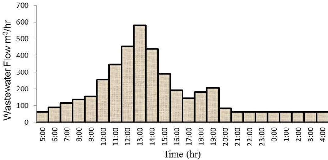
**Figure 17:** Average hourly wastewater flow for the main catchment on a non-working day in Nablus-East
