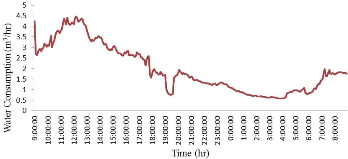
**Figure 11:** 24 hour’s water consumption for on a non-working day in the sub-main catchment in Nablus-East
