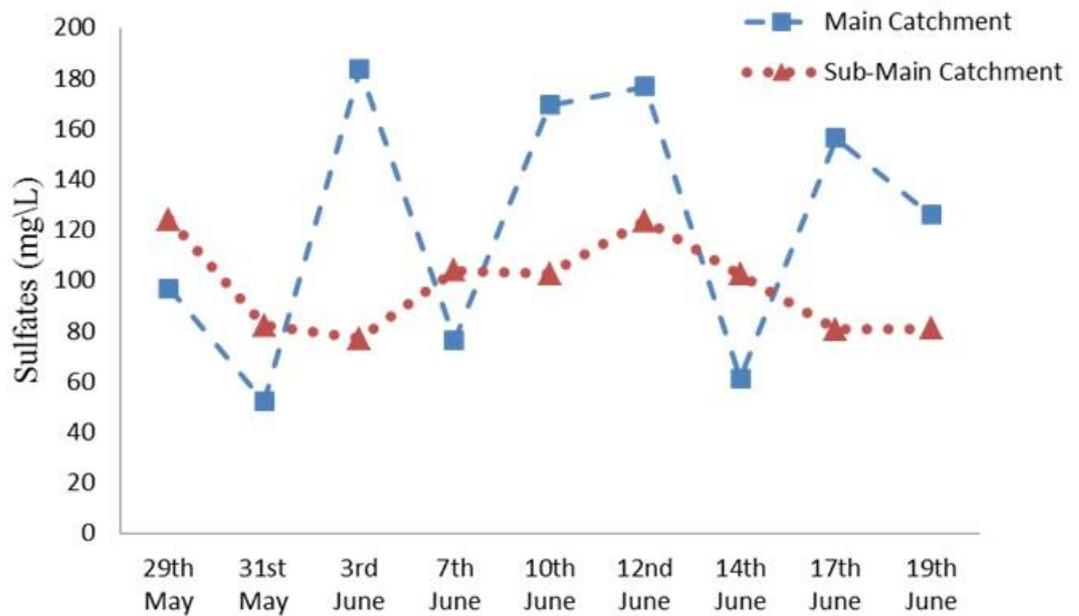
Figure 23: **Temporal variability of Sulfates values for the main and sub-main catchments**Figure 23 depicts the temporal variability of Sulfates values for the measured samples. The results show high variability between working days and non-working days in the main catchment.
