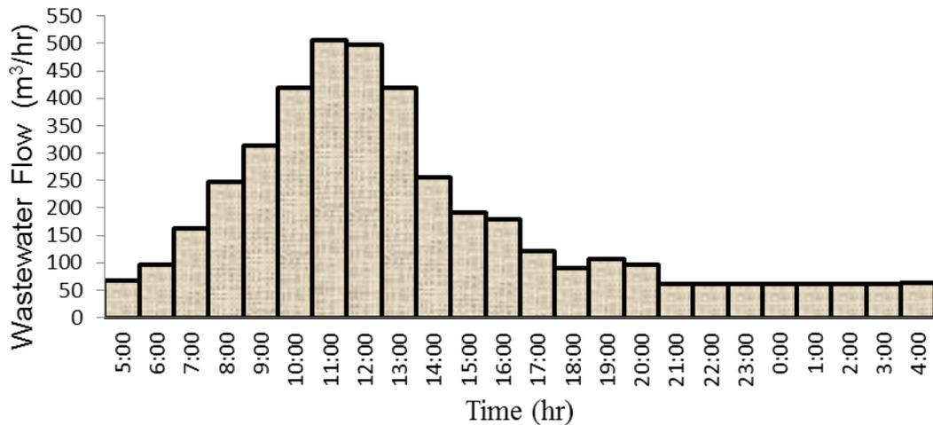
**Figure 16:** Average hourly wastewater flow on a working day for the main catchment in Nablus-East
