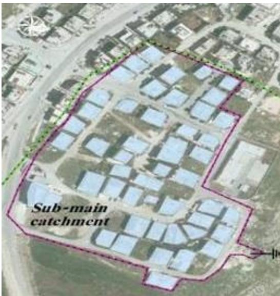
**Figure 4:** Sub catchment outlet and boundary
