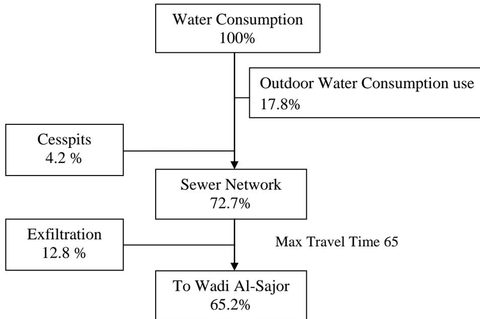
**Figure 18:** Water and wastewater mass balance for the main catchment in Nablus-East
