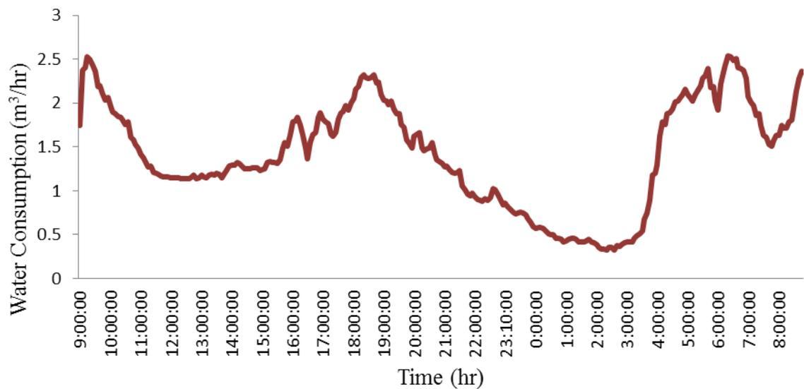
**Figure 12:** 24 hour’s water consumption on a working day in the sub-main catchment in Nablus-East
