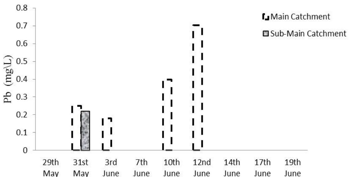
**Figure 28:** Temporal variability of Lead concentration for the main and sub-main catchments
