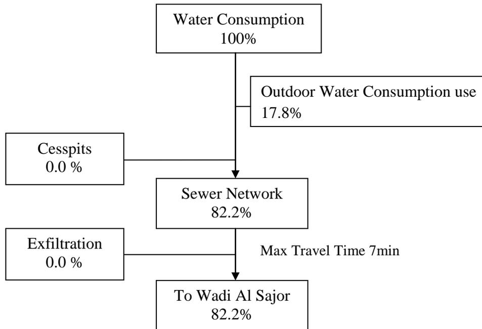
**Figure 15:** Water and wastewater mass balance for the sub-main catchment in Nablus-East
