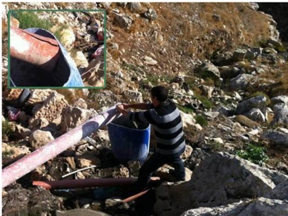
**Figure 9:** Sub-main catchment outlet sampling method in Nablus-East
