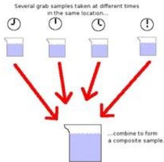
**Figure 1:** Composite sampling concept
