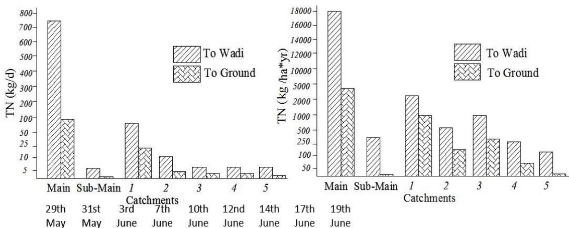
**Figure 32:** Nitrogen loading by catchments as absolute nitrogen loading (kg/day) and loading by area (kg/ha\* yr) from Nablus-East wastewater; 1-5: sub-catchments
