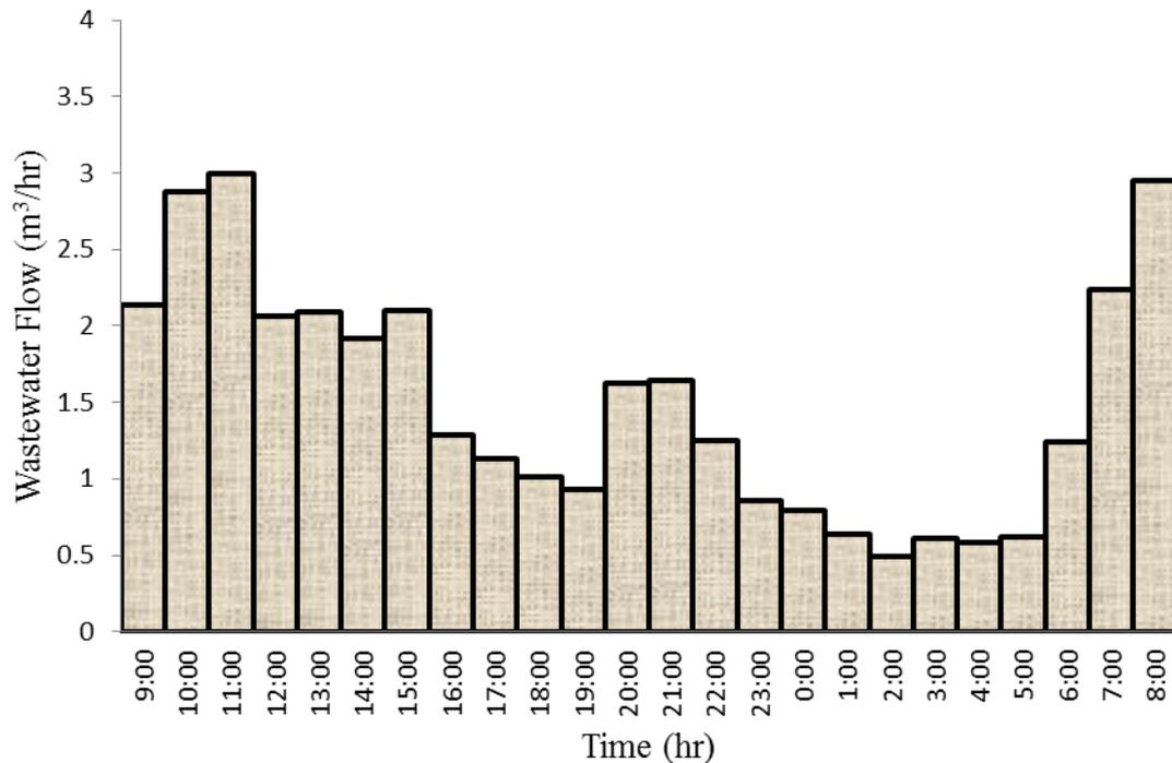
**Figure 13:** 24 hour's wastewater flow on a non-working day in the sub-main catchment in Nablus-East
