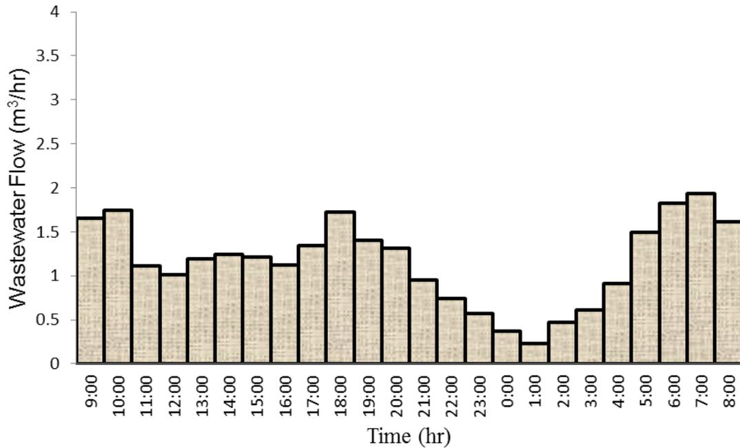
**Figure 14:** 24 hour's wastewater flow on a working day in the sub catchment in Nablus-East
