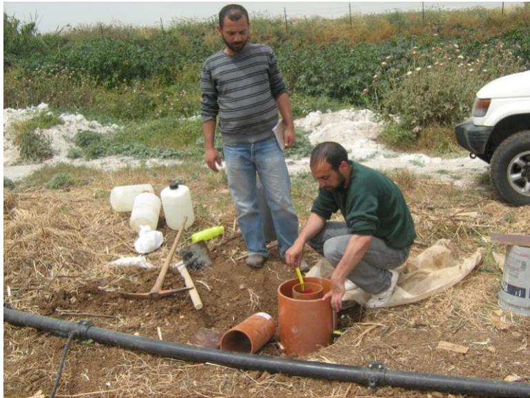
**Figure 3.4:** Infiltration test using double ring method
