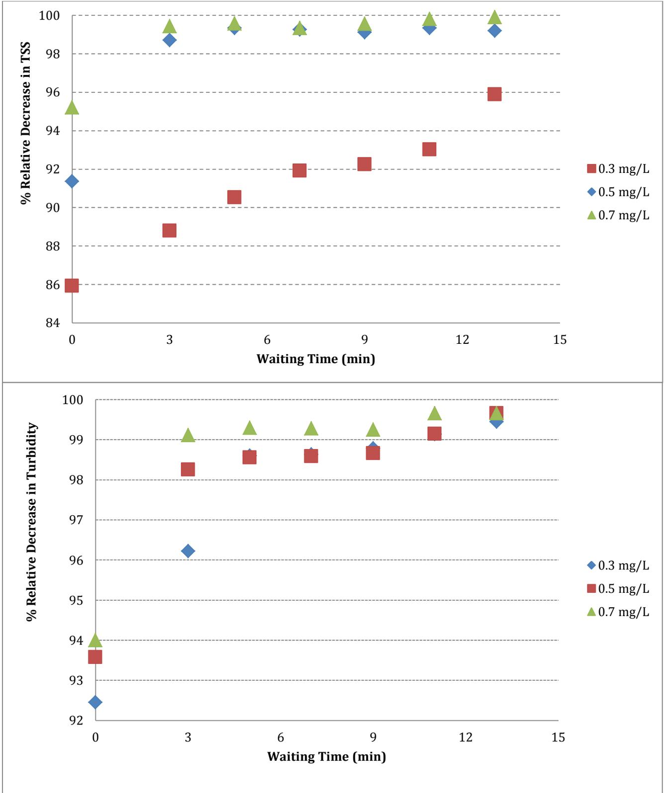
Figure 5.3: Percentage relative decrease in both of TSS and Turbidity as a function of waiting time for Coagulation experiments.
