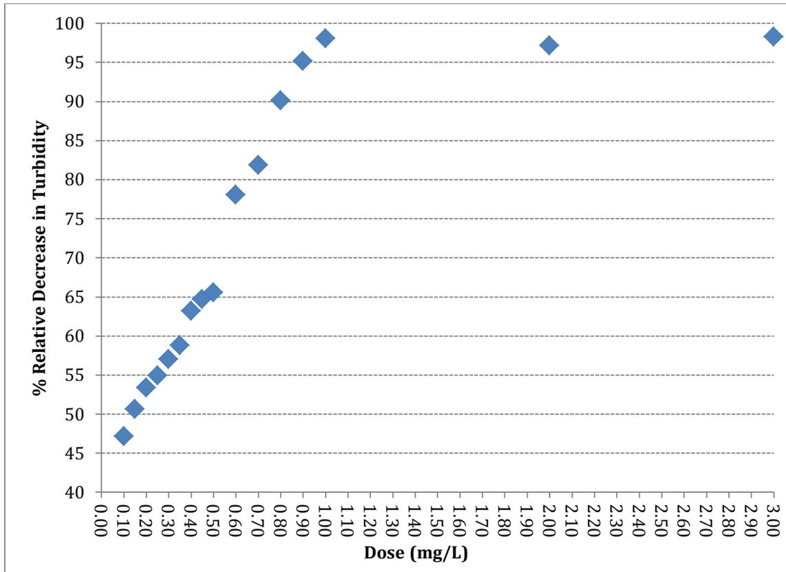
Figure 5. 5: Equilibrium percentage relative decrease in Turbidity as a function of dose of Ferric chloride.
