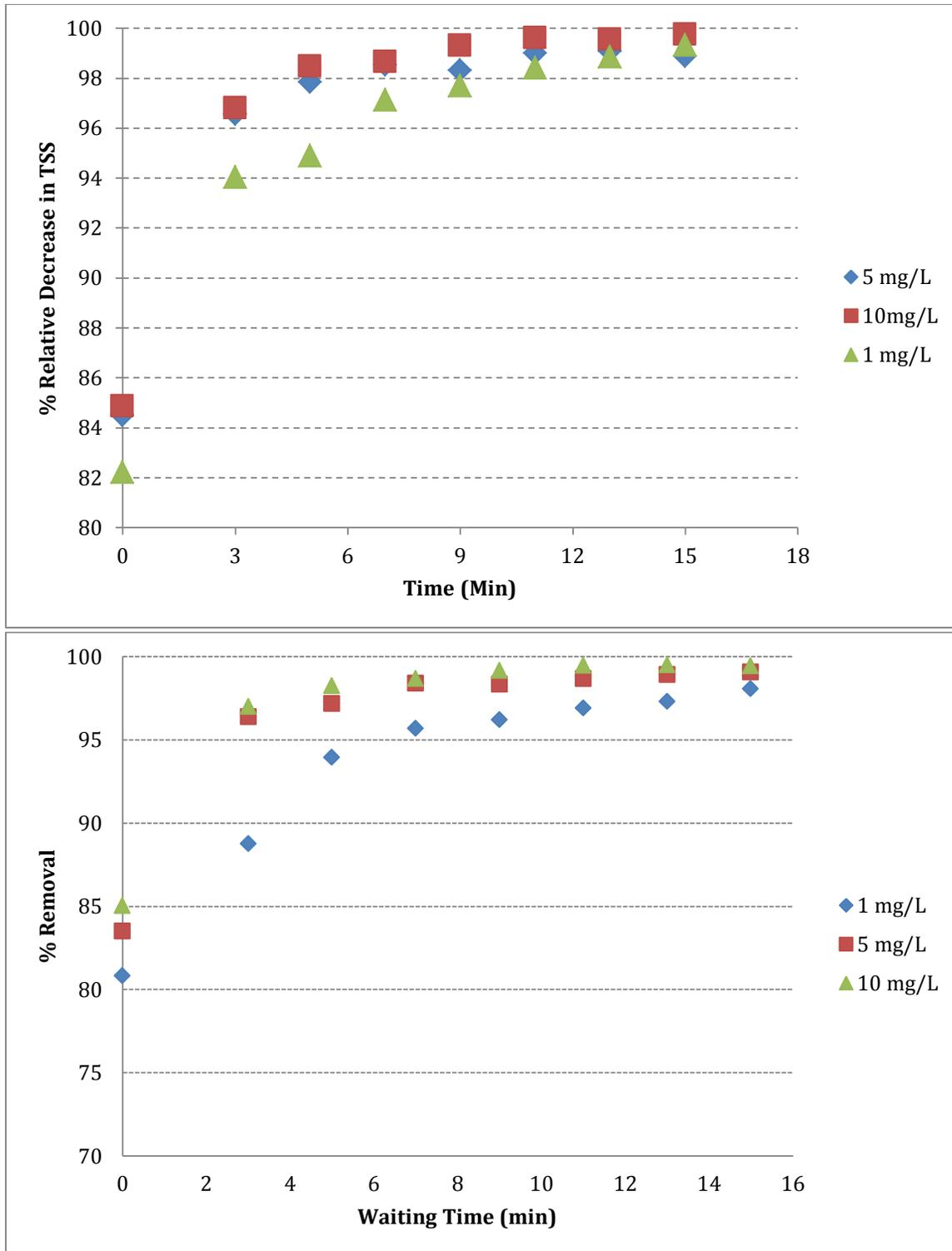
Figure 5. 6: Percentage relative decrease in both of TSS and Turbidity as a function of waiting time for Coagulation experiments.
