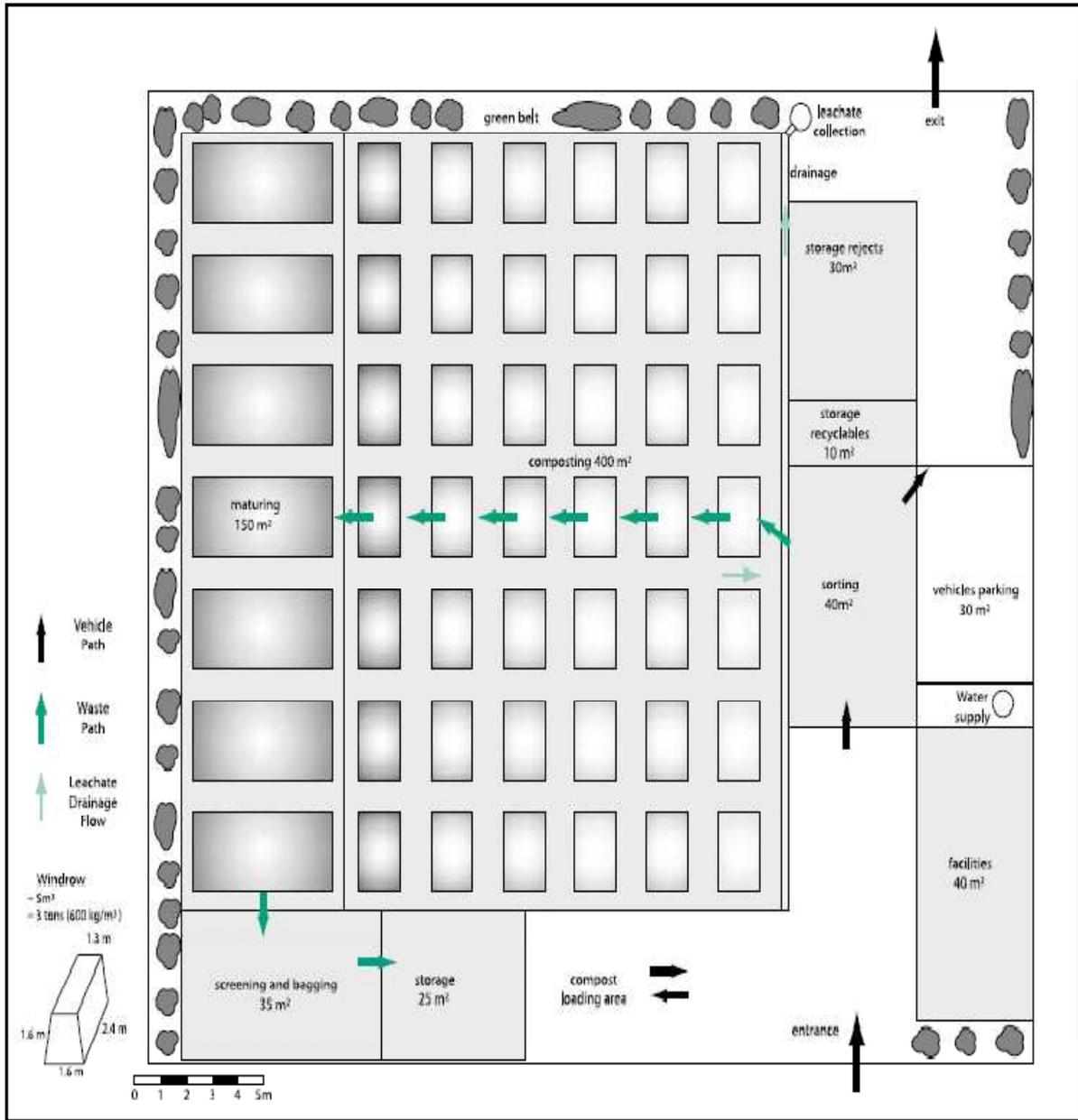
**Fig. 4.3:** Windrow-composting system layout plan (Rothenberger et al., 2006).
