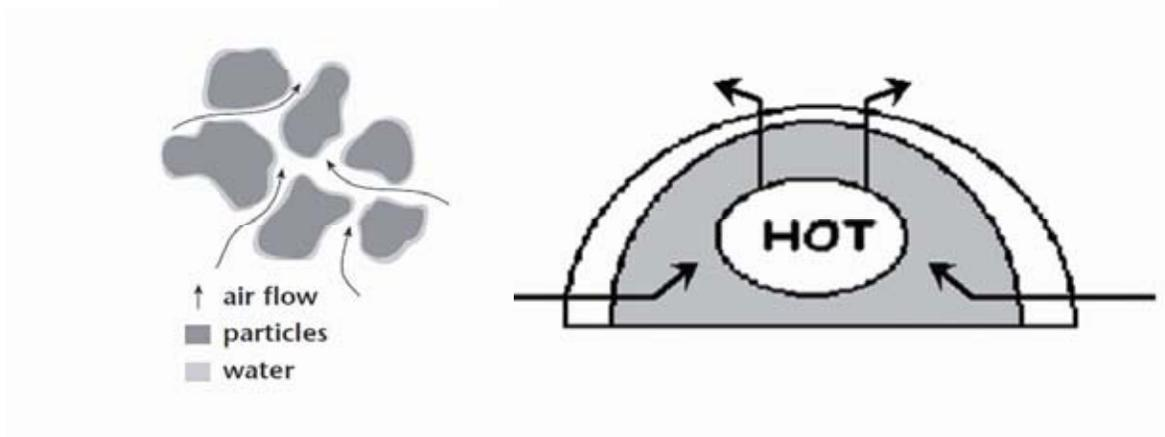
**Fig.2.3:** Air circulation in a compost pile (Schneider et al., 2001).
