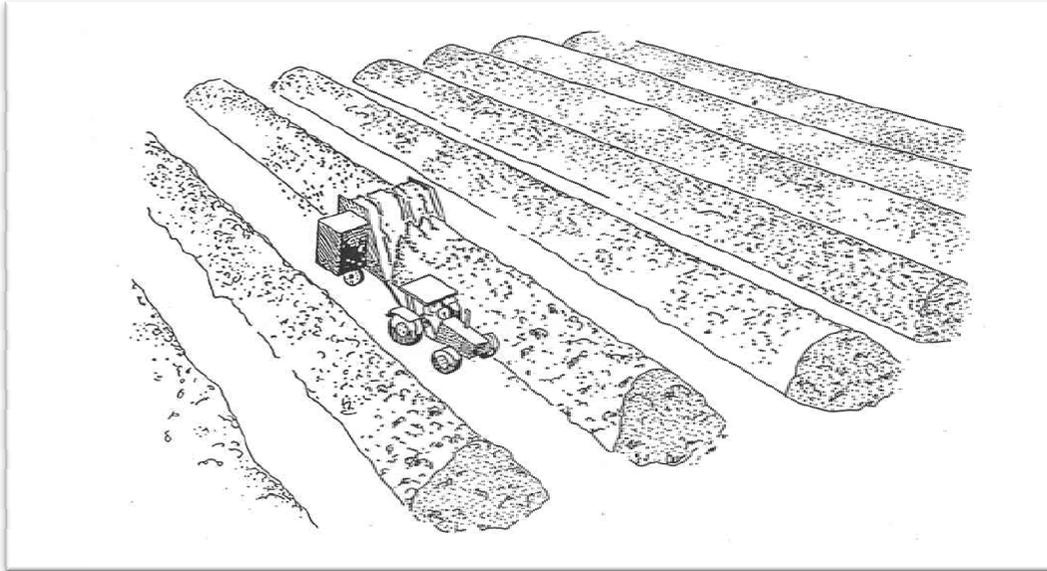
**Fig. 2.6:** Windrow composting(Schneider et al., 2001).
