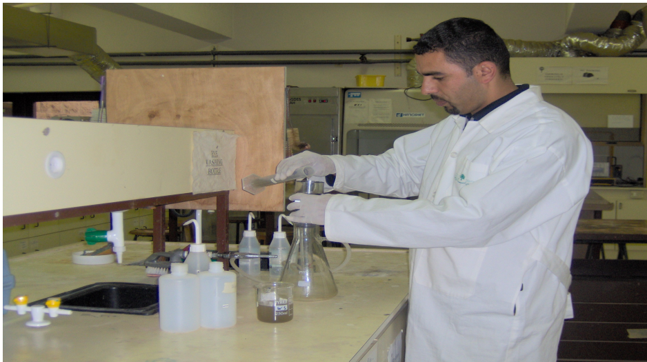
Photo 5. Membrane-filtered process for total coliform in Wastewater using 4.4- \mu\text{m} paper filters
