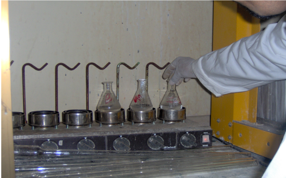
Photo 4. Digestion process for analysis of ammonia in wastewater
