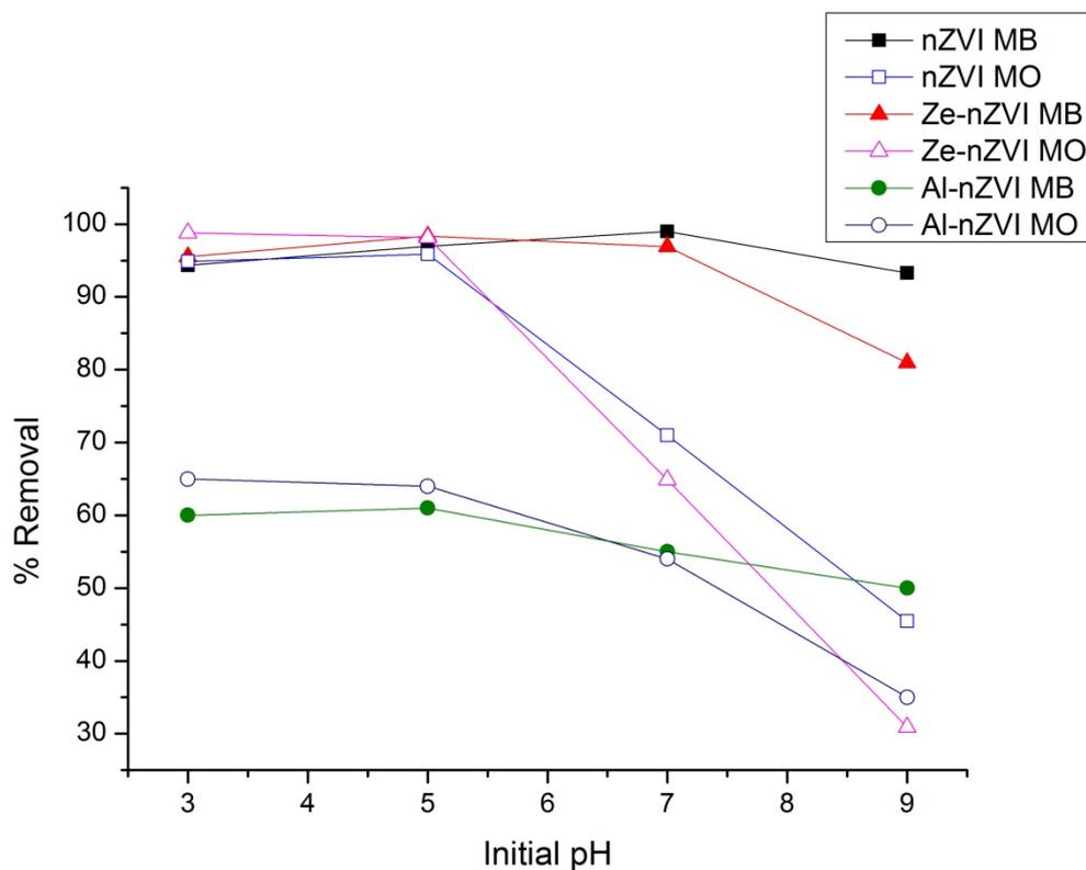
**Figure 3.48 Dye removal % at different initial pH values**
