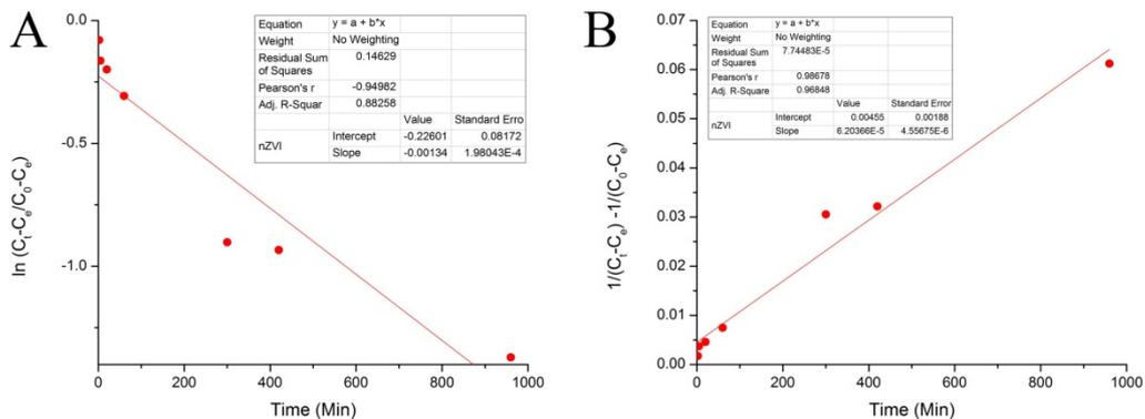
**Figure 3.56 First order (A) and second order (B) kinetics for the removal of 100 mg L<sup>-1</sup> MO using nZVI as a Fenton catalyst**
