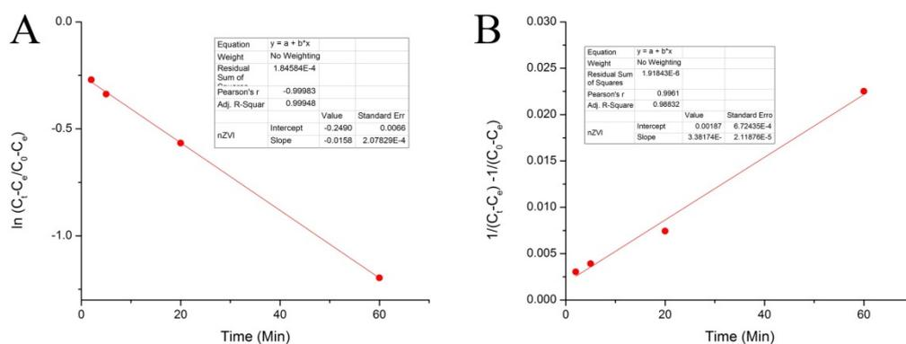
**Figure 3.53** First order (A), and second order (B) kinetics for the removal of  $100.0 \text{ mg L}^{-1}$  MB using nZVI as a Fenton catalyst
