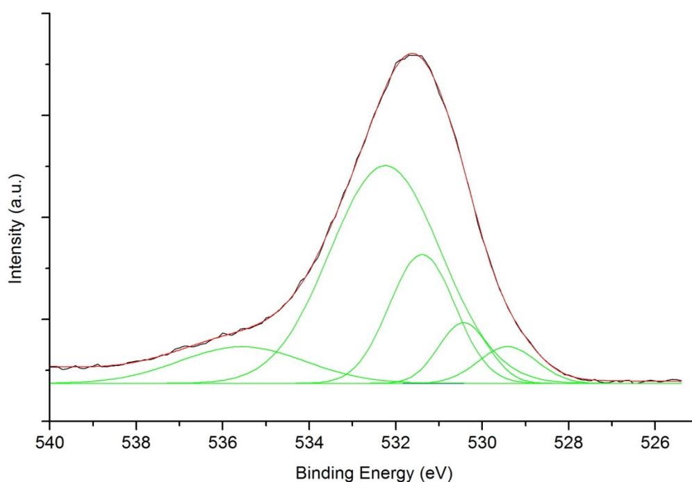
**Figure 3.40 O 1s photoelectron peak with curve fitting**
