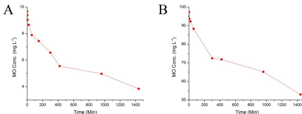
**Figure 3.54** MO removal using nZVI as a Fenton catalyst at 10.0 mg L<sup>-1</sup> (A), and 100.0 mg L<sup>-1</sup> (B)
