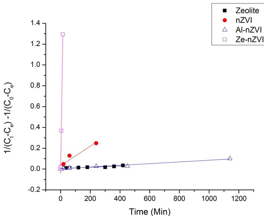
Figure 3.44 Second order linear fit for the removal of MB at initial concentration of  $100.0 \text{ mg L}^{-1}$
