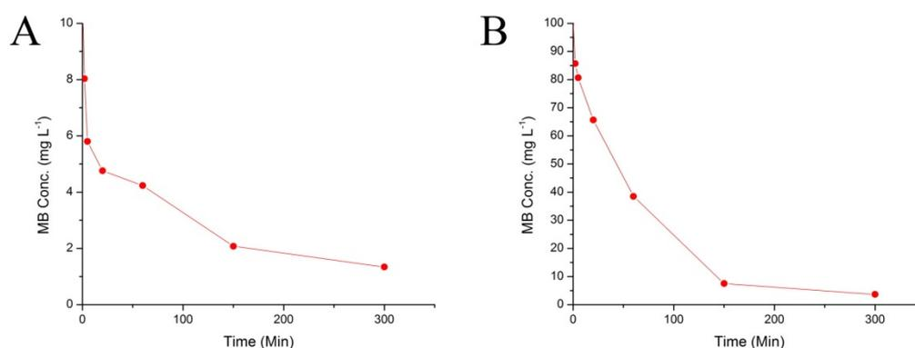
**Figure 3.51 MB removal using nZVI as a Fenton catalyst at 10.0 mg L<sup>-1</sup> (A), and 100.0 mg L<sup>-1</sup> (B)**
