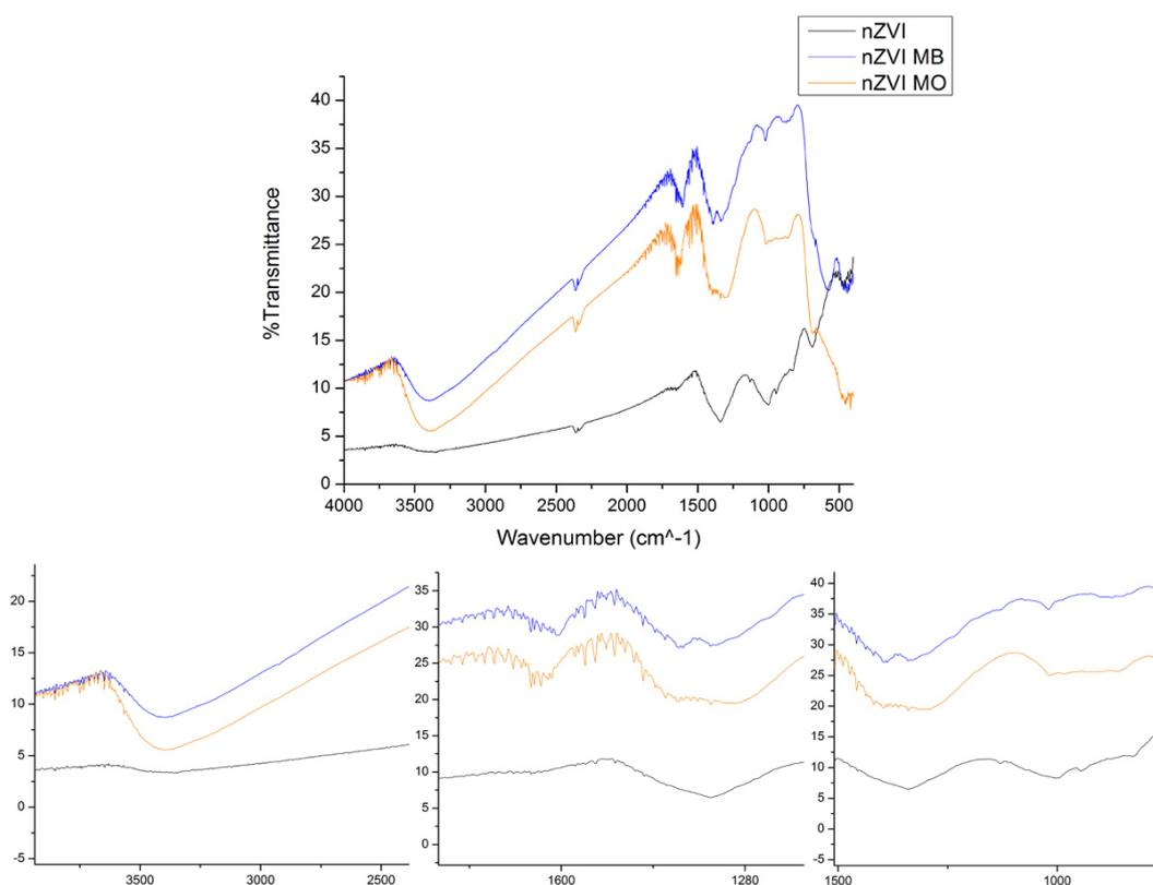
**Figure 3.7 FTIR spectra of nZVI, nZVI MB and nZVI MO**
