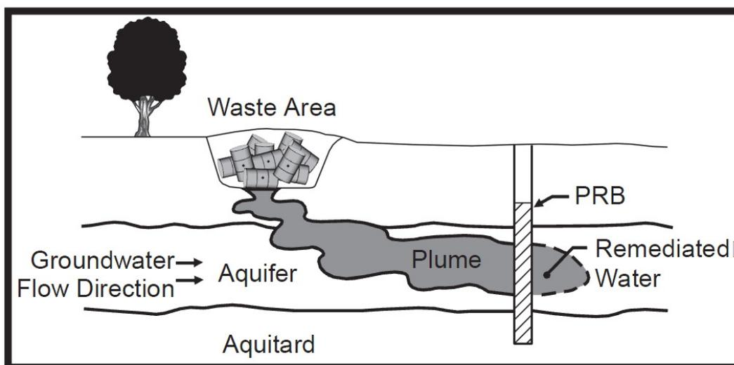
Figure 1.3 A typical diagram of Permeable reactive barrier (PRB)<sup>28</sup>
