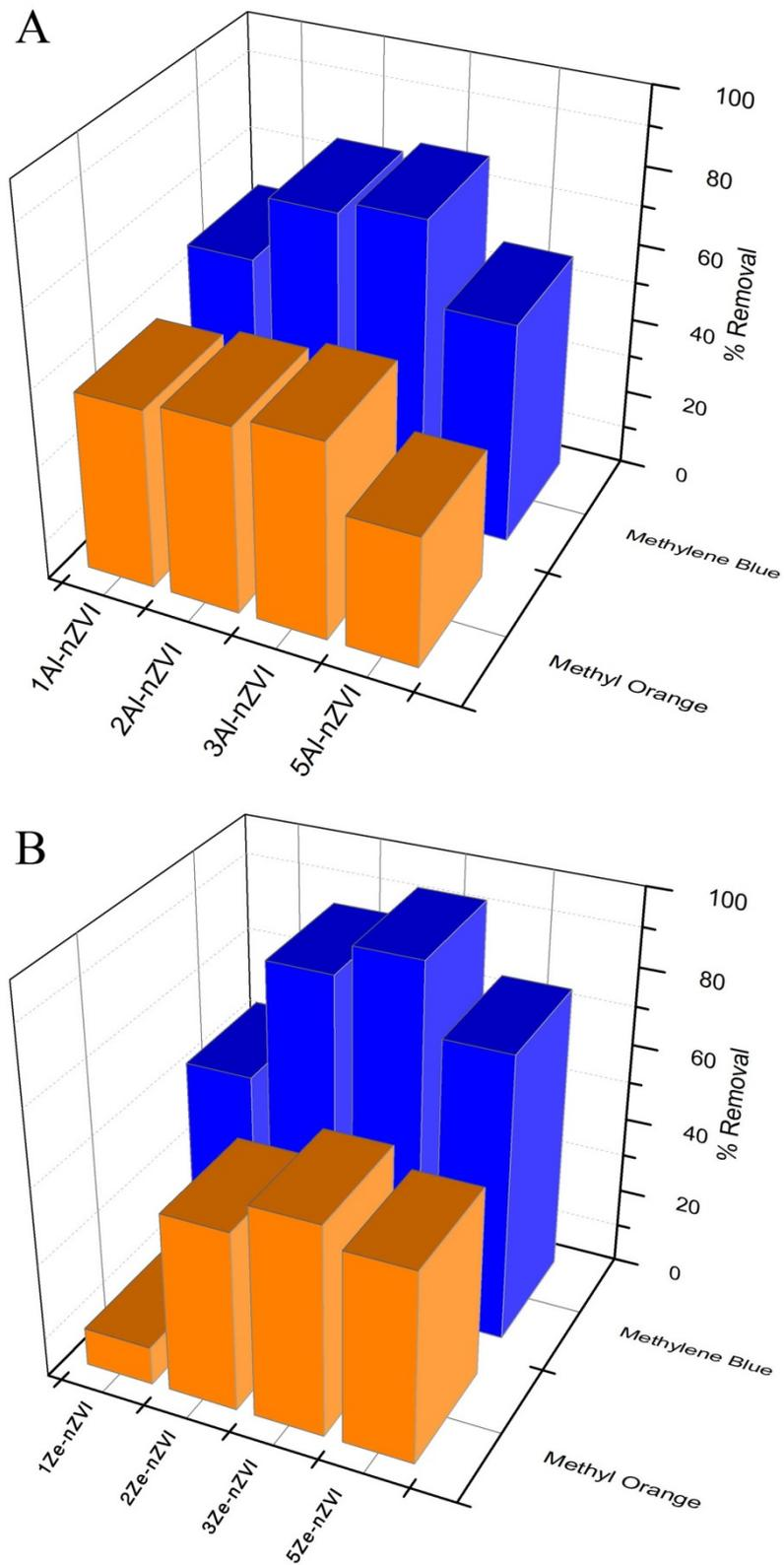
**Figure 3.41 MB and MO removal using different alumina:nZVI (A) and zeolite:nZVI (B) ratios**
