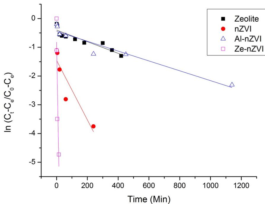
**Figure 3.43 First order linear fit for the removal of MB at initial concentration of  $100.0 \text{ mg L}^{-1}$**
