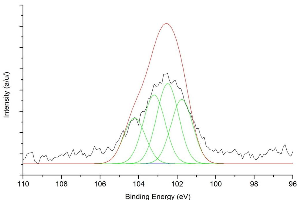
**Figure 3.39 Si 2p photoelectron peak with curve fitting**
