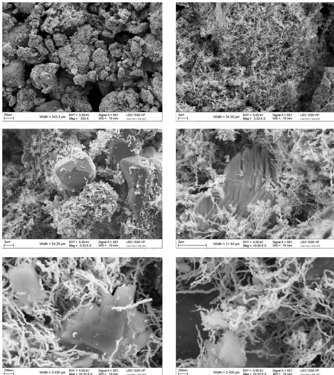
**Figure 3.31 SEM images of Ze-nZVI at various magnifications**
