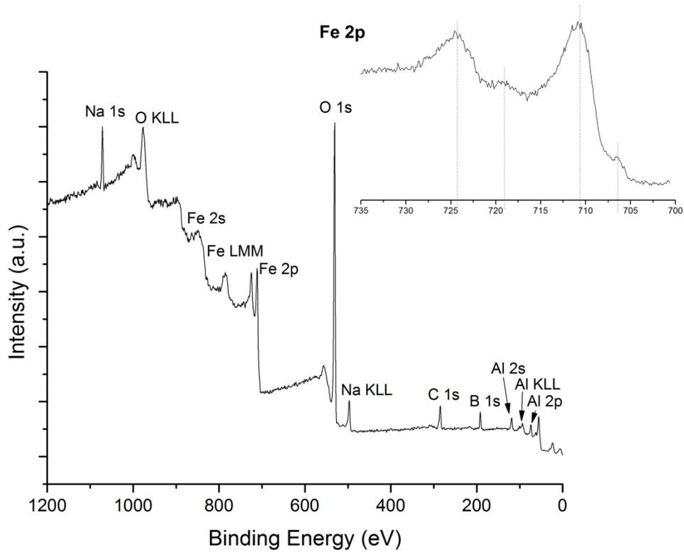
**Figure 3.24 XPS spectrum of Al-nZVI with an inset of Fe2p**
