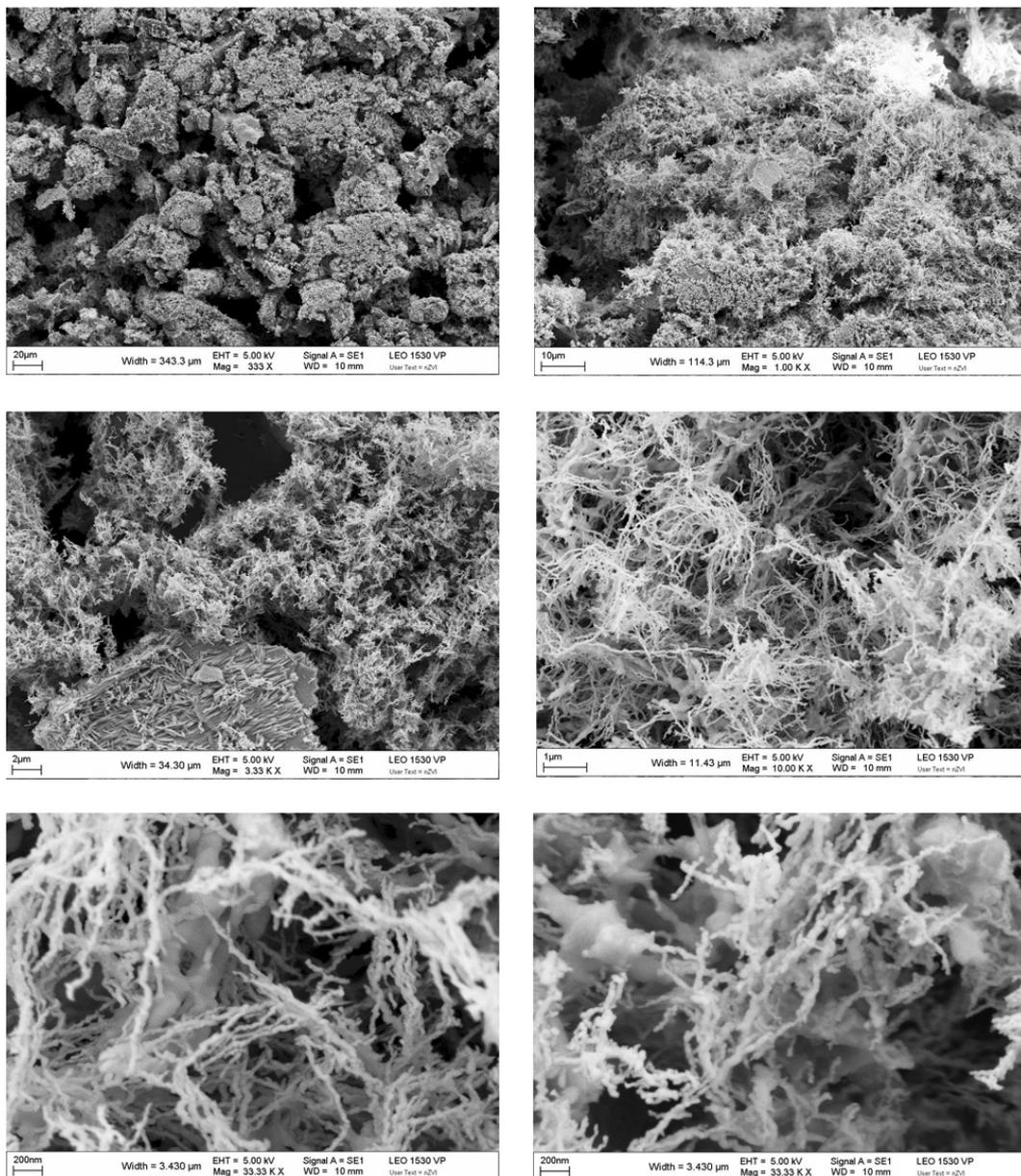
**Figure 3.9 SEM images of nZVI at various magnifications**
