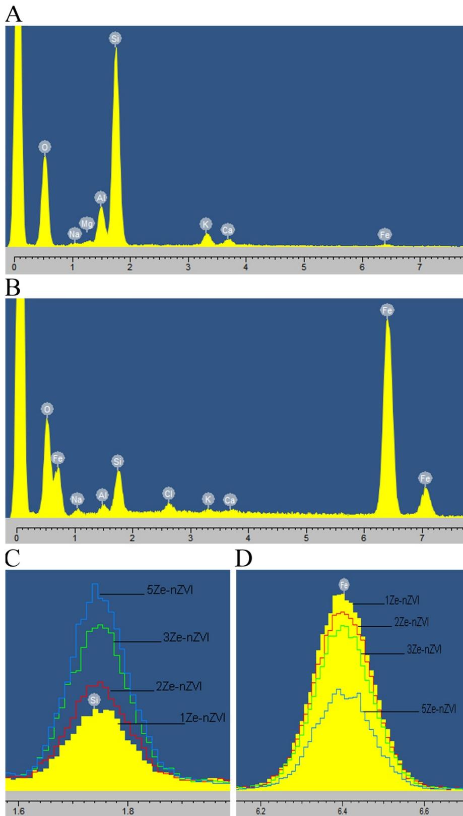
**Figure 3.33** EDX spectra of zeolite (A), Ze-nZVI (B), Si peak in Ze-nZVI (C) Fe peak in Ze-nZVI (D)
