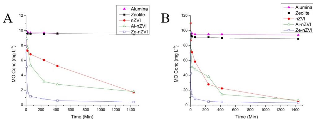
**Figure 3.45** MO removal at initial conc. 10.0 mg L<sup>-1</sup> (A), and 100.0 mg L<sup>-1</sup> (B)
