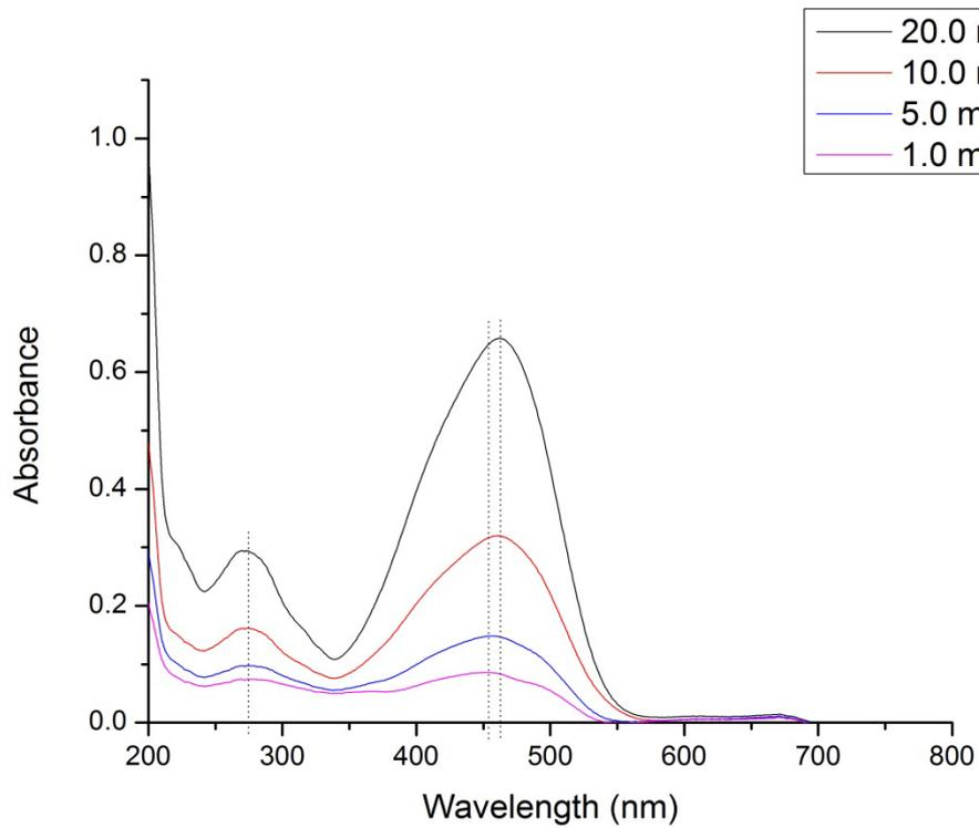
**Figure 3.2 Various MO concentrations absorbance spectra**
