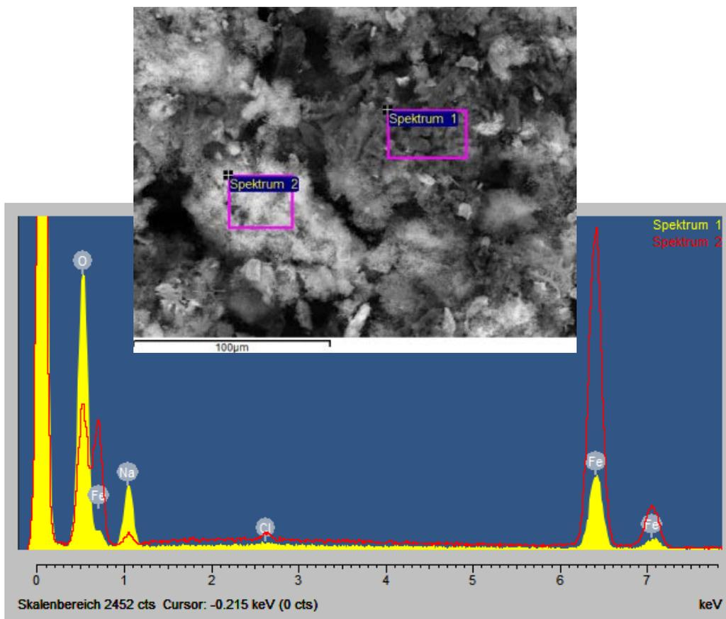
**Figure 3.11 Selected areas EDX spectra of a back-scattered SEM**
