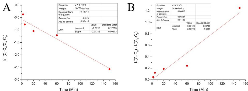
**Figure 3.52** First order (A), and second order (B) kinetics for the removal of  $10.0 \text{ mg L}^{-1}$  MB using nZVI as a Fenton catalyst
