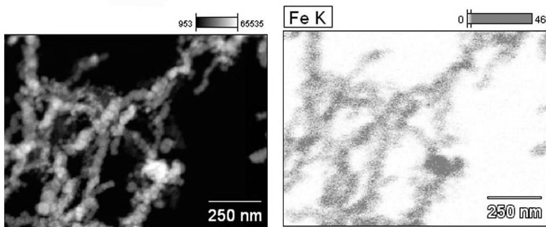
**Figure 3.23 Al-nZVI STEM image and its EDX Fe mapping**
