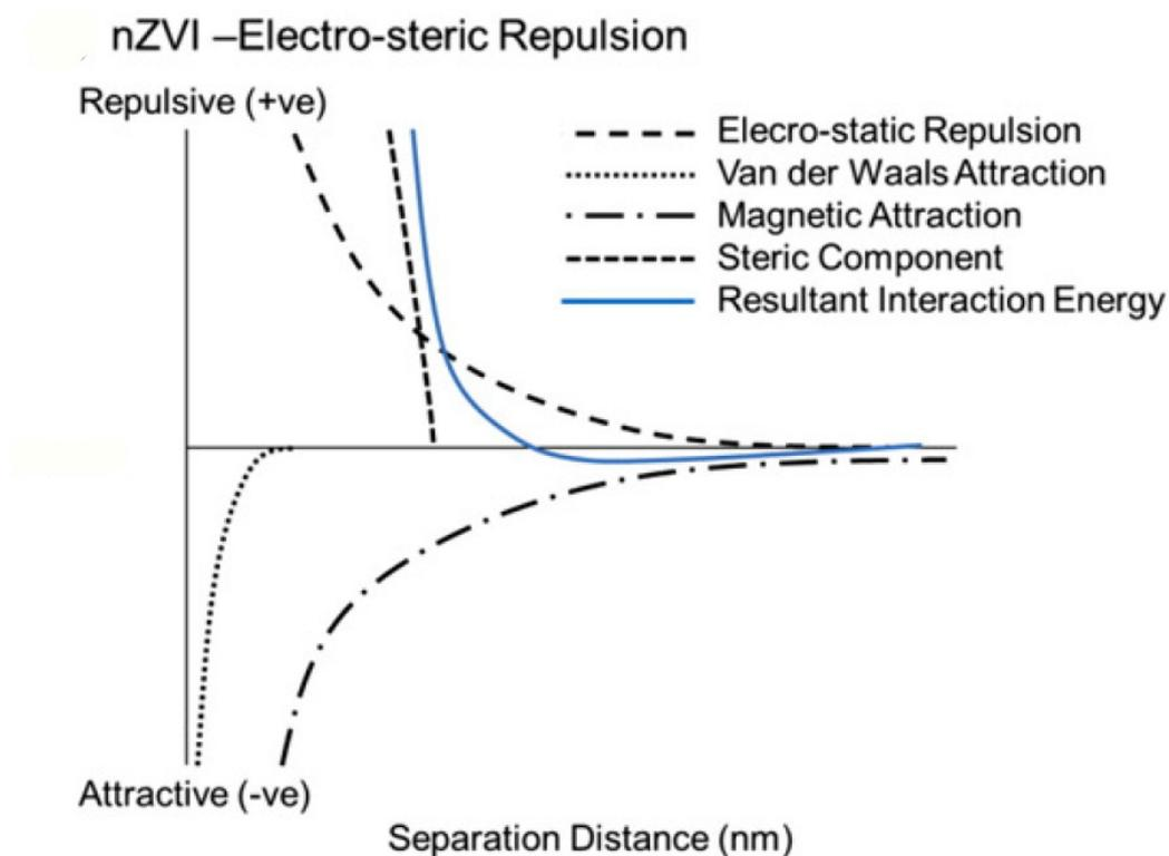
**Figure 1.6 Conceptual model of DLVO interaction forces for stabilized nZVI particles.**<sup>44</sup>
