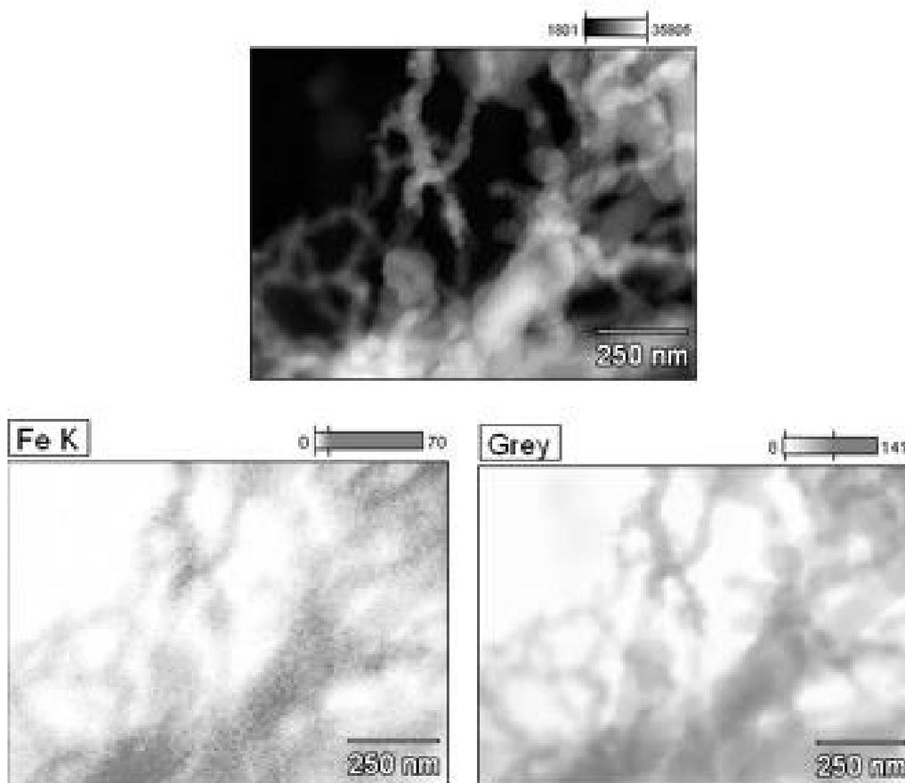
**Figure 3.15 nZVI STEM image and Fe EDX mapping**
