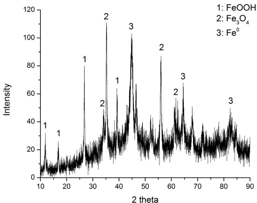
**Figure 3.8 XRD pattern of nZVI showing crystalline iron along with iron (hydr)oxides**
