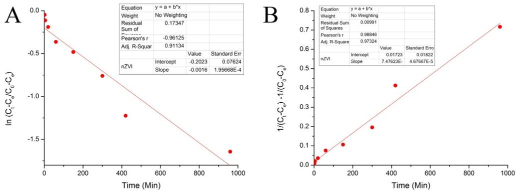
**Figure 3.55 First order (A). and second order (B) kinetics for the removal of 10 mg L<sup>-1</sup> MO using nZVI as a Fenton catalyst**
