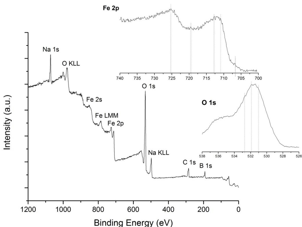
**Figure 3.16 XPS spectrum of nZVI with an inset of Fe2p and O1s peaks**
