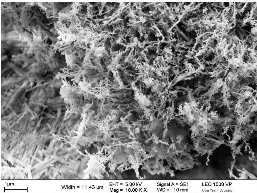
**Figure 3.19 SEM images of Al-nZVI at various magnifications**
