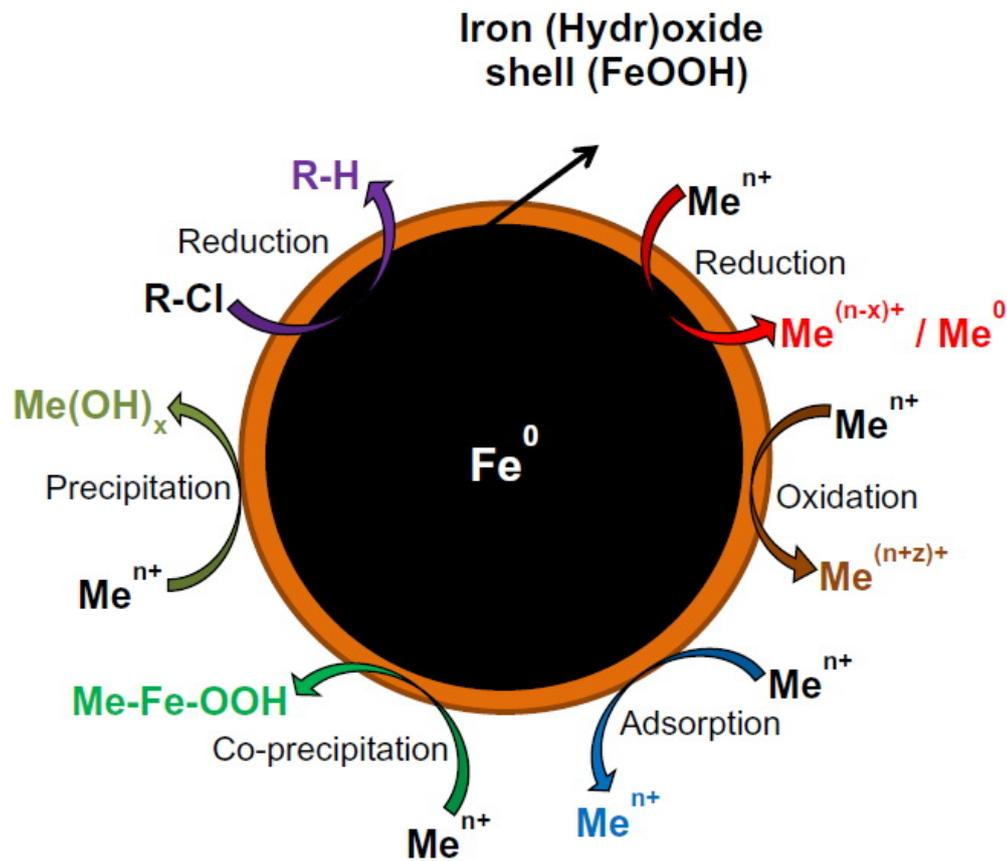
Figure 1.4 nZVI core shell structure showing various contaminants removal/degradation mechanisms.<sup>44</sup>
