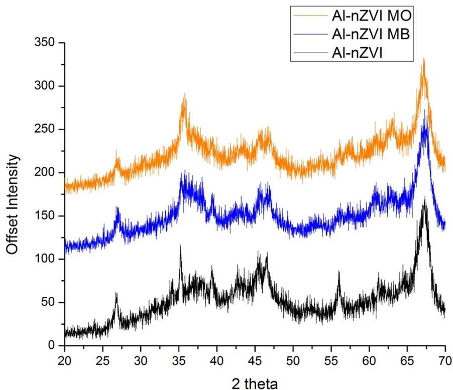
**Figure 3.18 XRD patterns of Al-nZVI, Al-nZVI MB and Al-nZVI MO**
