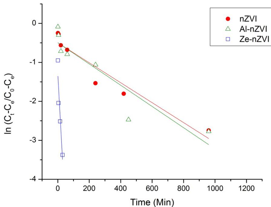
**Figure 3.46** First order linear fit for the removal of MO at  $100.0 \text{ mg L}^{-1}$
