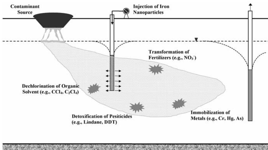
Figure 1.2 *In-situ* water treatment via direct injection<sup>25</sup>
