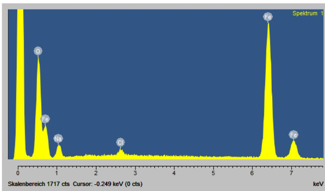
**Figure 3.10** EDX spectrum of nZVI
