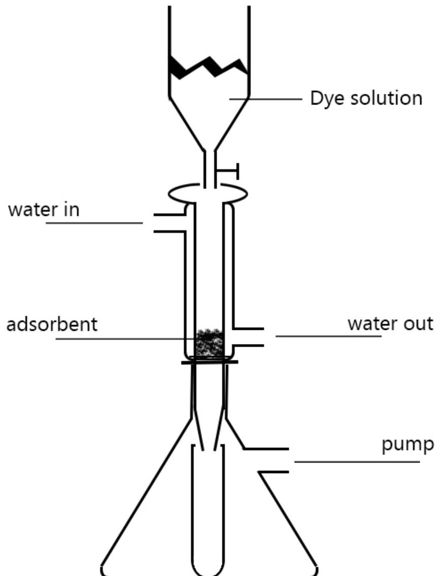
**Figure 2.2 Glass column for dye removal using a continuous flow system**
