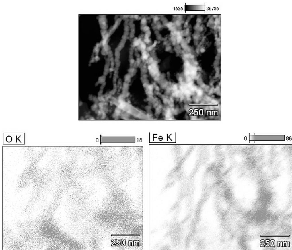
**Figure 3.36 STEM image of Ze-nZVI and elemental mappings for O and Fe**
