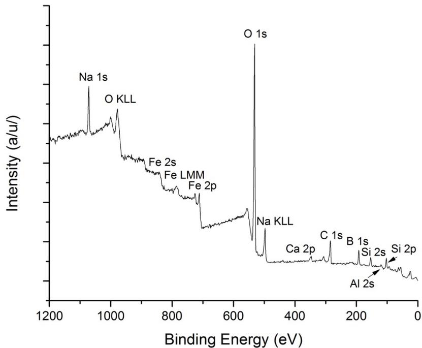
**Figure 3.37 XPS spectrum of Ze-nZVI**
