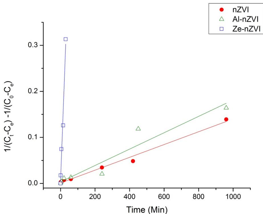
Figure 3.47 Second order linear fit for the removal of MO at 100.0 mg L<sup>-1</sup>
