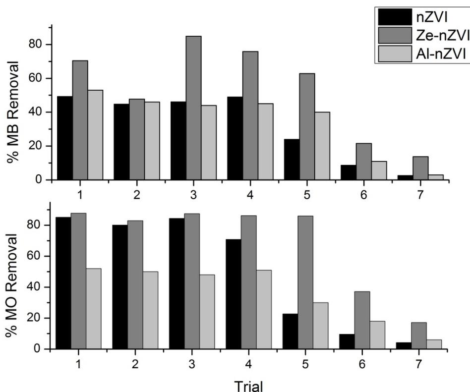
Figure 3.49 Reusability of nZVI, Al-nZVI and Ze-nZVI in dye removal
