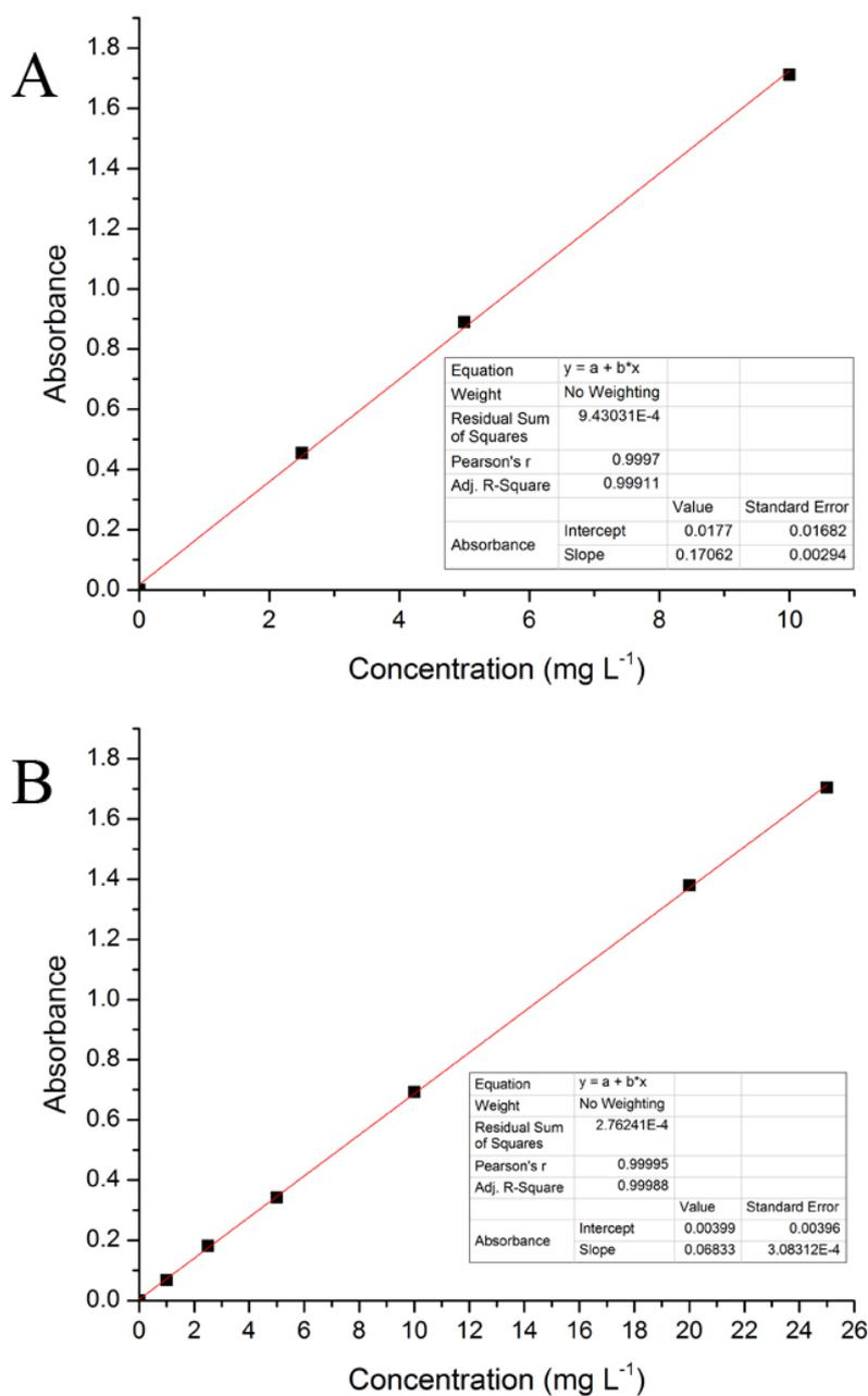
**Figure 2.3 Standard calibration curves for MB (A) and MO (B)**
