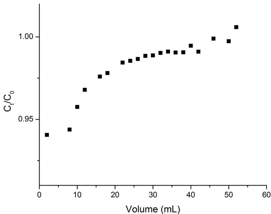
**Figure 3.57 Breakthrough curve for the removal of MB using alumina**
