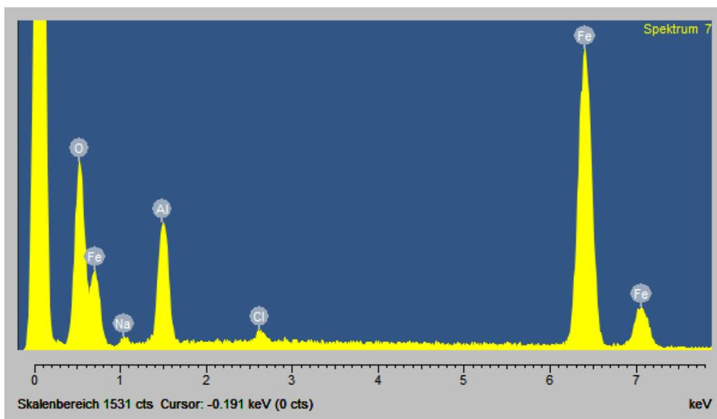
**Figure 3.21** EDX spectrum of Al-nZVI
