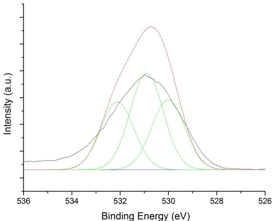
**Figure 3.26 O 1s photoelectron peak with curve fitting**
