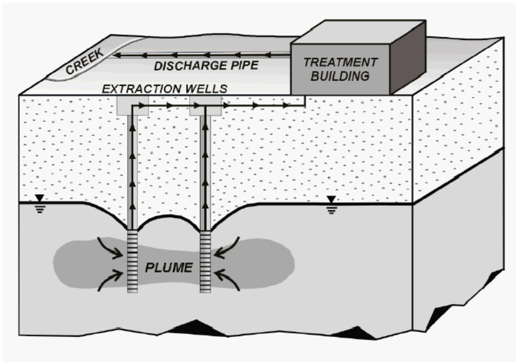
Figure 1.1 A typical diagram of Pump and treat system (PTS)<sup>22</sup>
