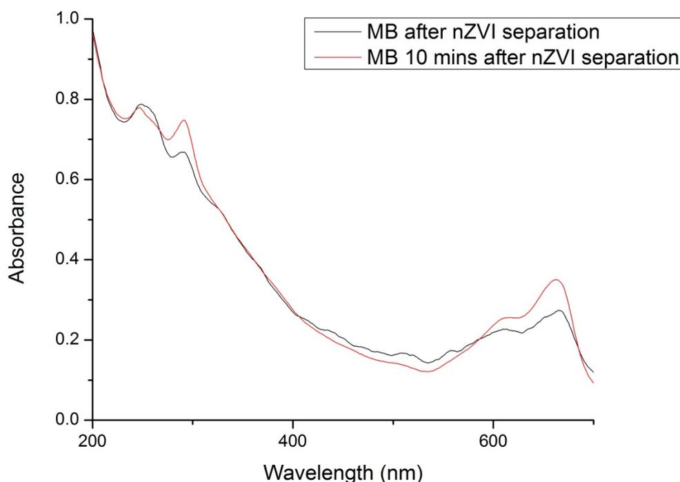
**Figure 3.5 MB spectra after nZVI separation**
