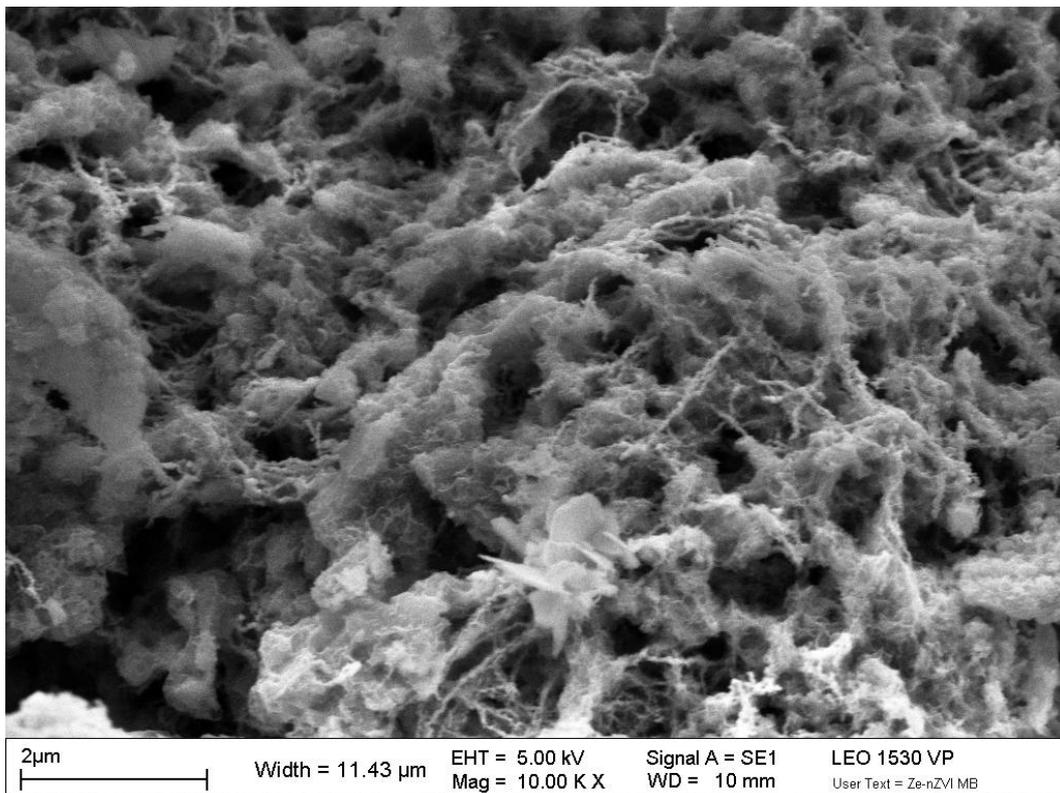
**Figure 3.34 SEM image of Ze-nZVI sample used in the removal of MB**
