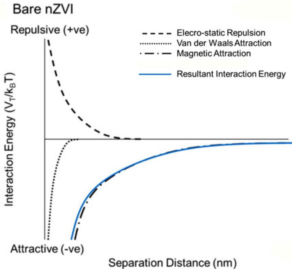
**Figure 1.5 Conceptual model of DLVO interaction forces for nZVI particles**
