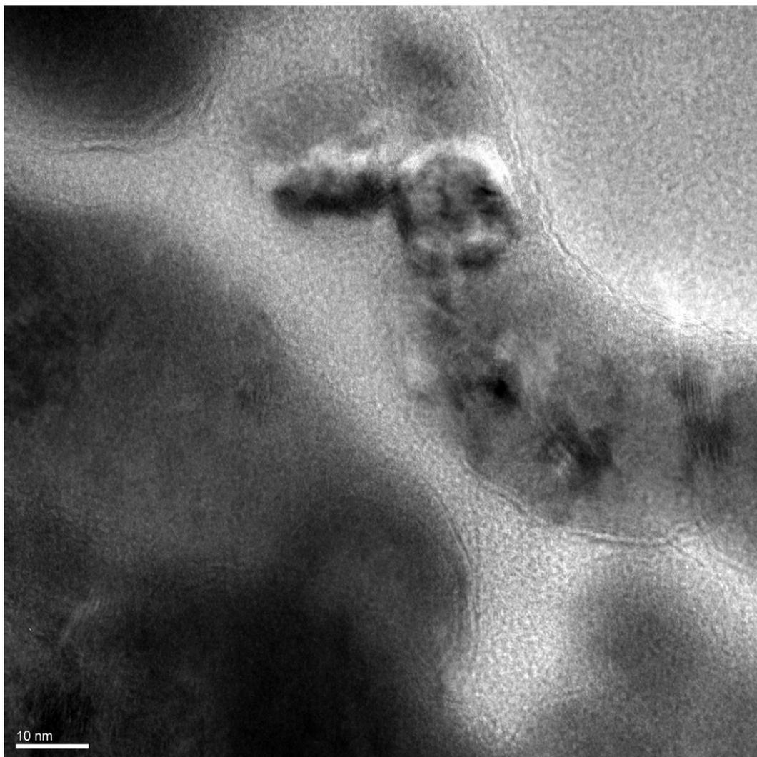
**Figure 3.14 HR-TEM of nZVI showing the core-shell structure**
