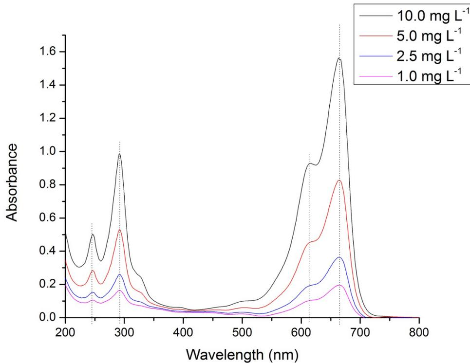
**Figure 3.1 Various MB concentrations absorbance spectra**
