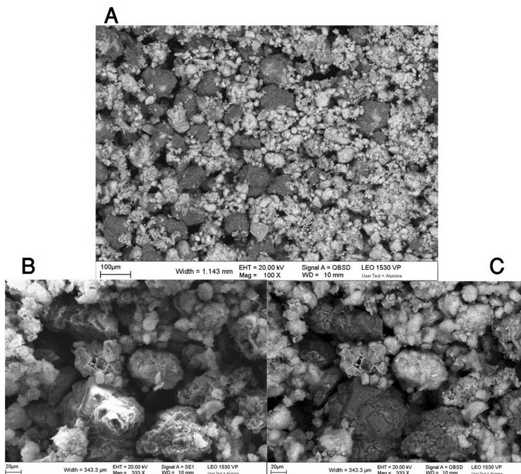
**Figure 3.20 Al-nZVI back-scattered SEM (A & C) and SEM (B)**
