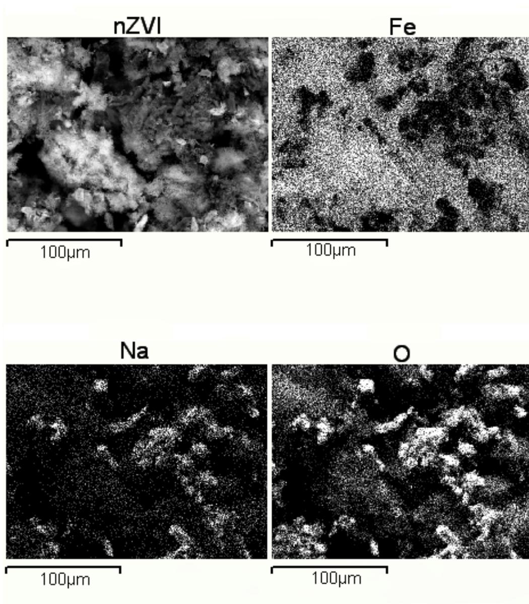
**Figure 3.12** EDX mappings of nZVI showing elemental maps for Fe, O and Na
