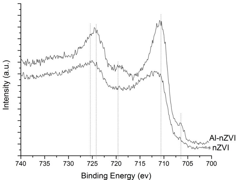
**Figure 3.25 Fe 2p photoelectron peaks of nZVI and Al-nZVI**
