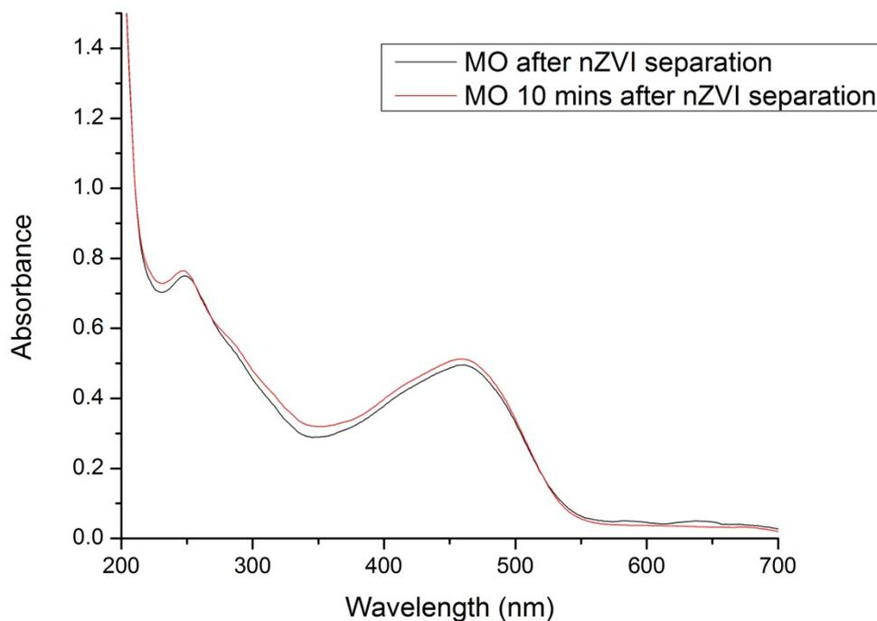
**Figure 3.6 MO spectra after nZVI separation**
