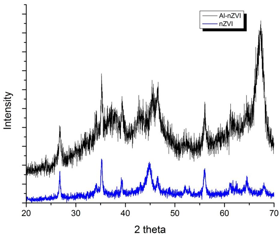
**Figure 3.17 XRD patterns for Al-nZVI and nZVI**
