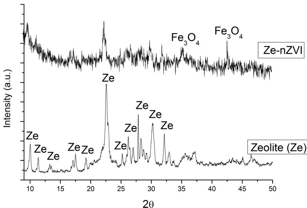
**Figure 3.29 XRD patterns of zeolite and Ze-nZVI**
