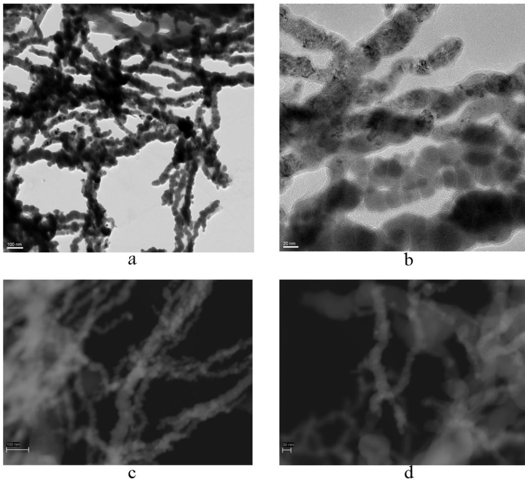
**Figure 3.13 nZVI TEM images (a and b) and STEM images (c and d)**
