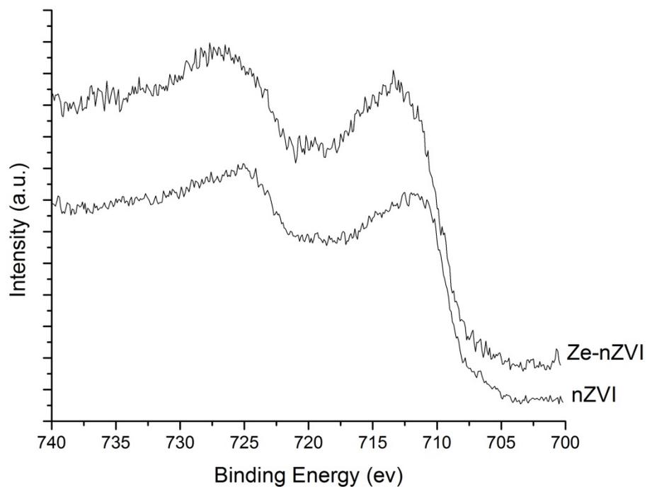
**Figure 3.38 Fe 2p photoelectron peaks of nZVI and Ze-nZVI**
