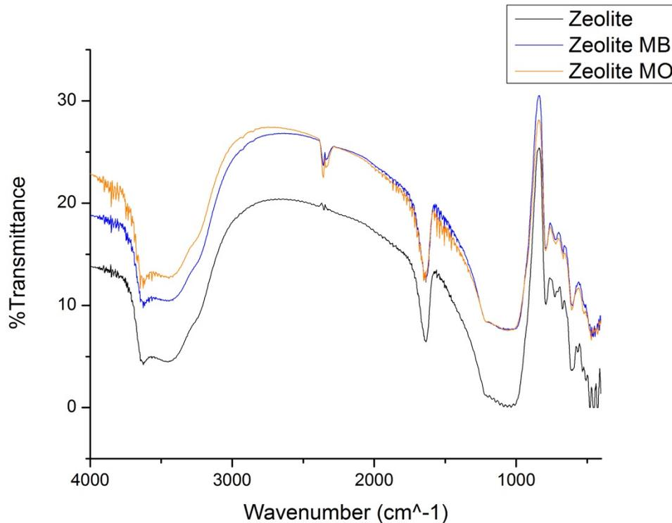
**Figure 3.27 FTIR spectra of zeolite, zeolite MB and zeolite MO**
