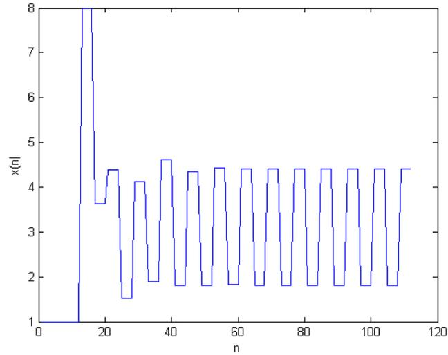
Figure 6.1: The Behavior of the Equilibrium point of the Equation  $x_n = \frac{5}{x_{n-4}} + \frac{3}{x_{n-12}}$
