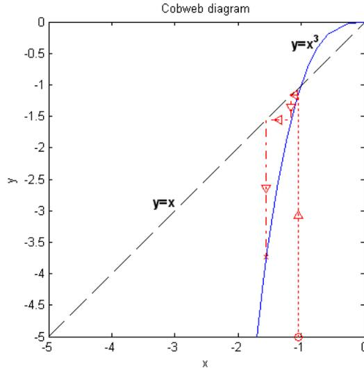
Figure 2.6: Stability of  $\bar{x} = -1$  of  $x(n + 1) = x^3(n)$
