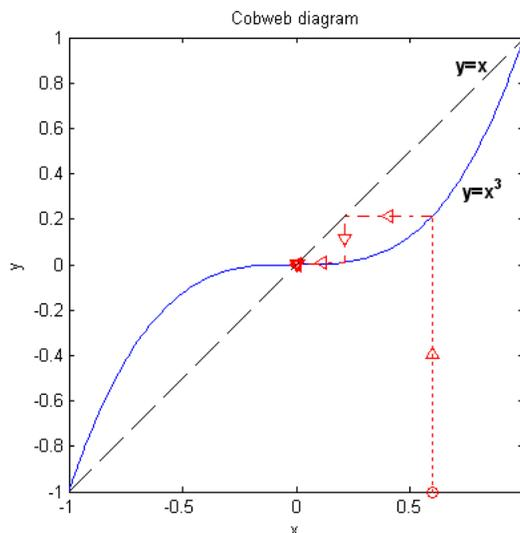
Figure 2.5: Stability of  $\bar{x} = 0$  of  $x(n + 1) = x^3(n)$
