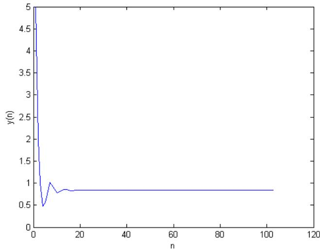
Figure 4.1: The Behavior of the Equilibrium point of the Equation  $y_{n+1} = \frac{0.5+y_n+0.5y_{n-2}}{y_n+1.5y_{n-2}}$
