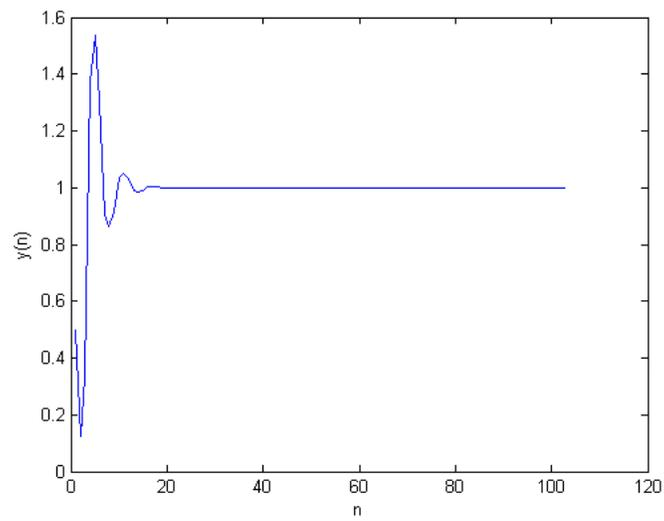
Figure 4.3: The Behavior of the Equilibrium point of the Equation  $y_{n+1} = \frac{1+y_n+y_{n-2}}{y_n+2y_{n-2}}$
